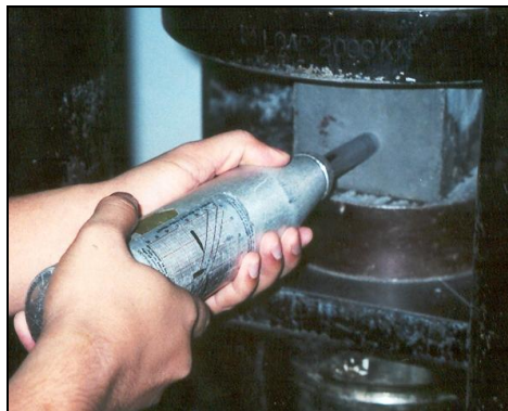
Figure 3.5: Rebound hammer test
