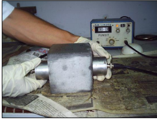
Figure 3.6: Ultrasonic pulse velocity (UPV) test
