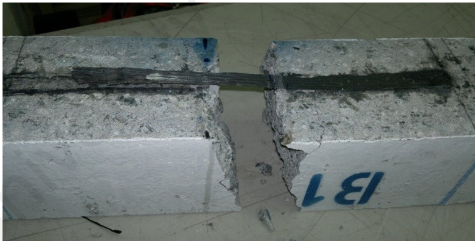
Figure 4.7: Separation of CFRP sheet in specimen B1
