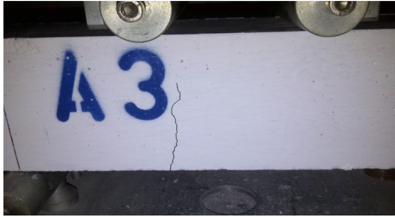
Figure 4.14: Propagation of crack in specimen A3 during test
