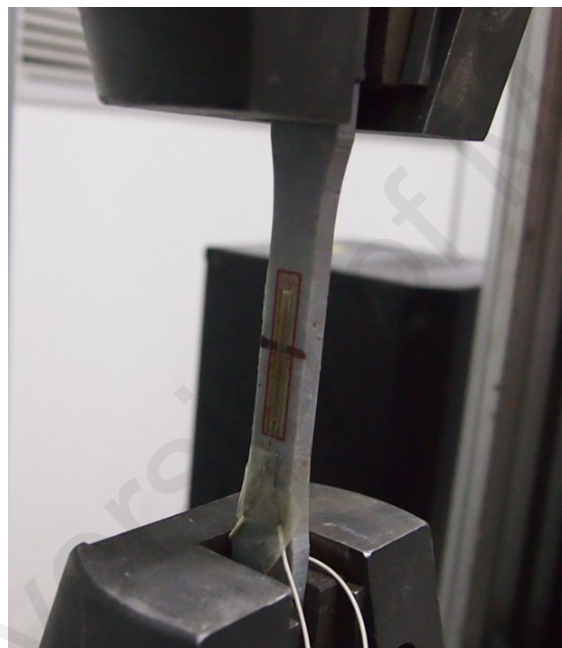
Figure B.10: Tensile test of epoxy resin
