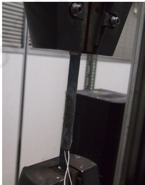
Figure B.8: Tensile test of CFRP sheet
