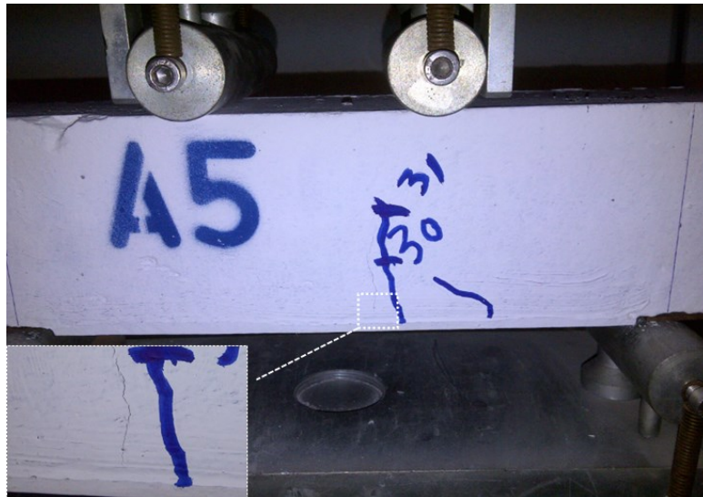
Figure 4.2: Crack propagation in A5 specimen during test
