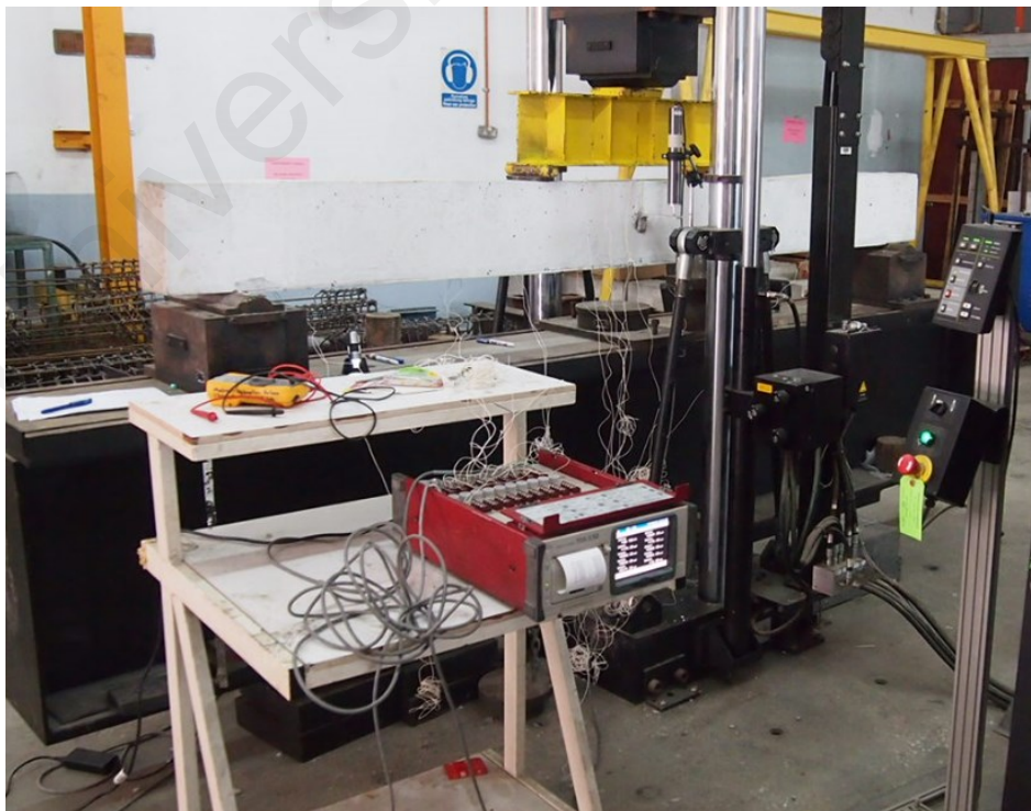
Figure 3.16: Test set-up of RC beams
