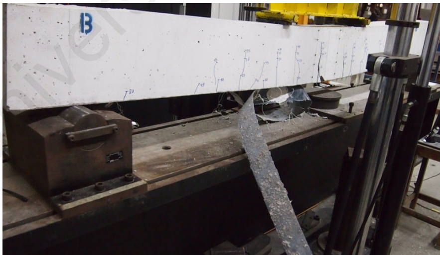
Figure 4.19: Debonding of CFRP sheet in specimen B
