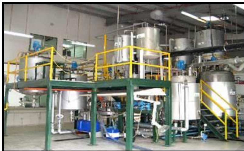
Figure 3.3: MPOB Pilot Plant Polyol with 500 kg production per batch.
