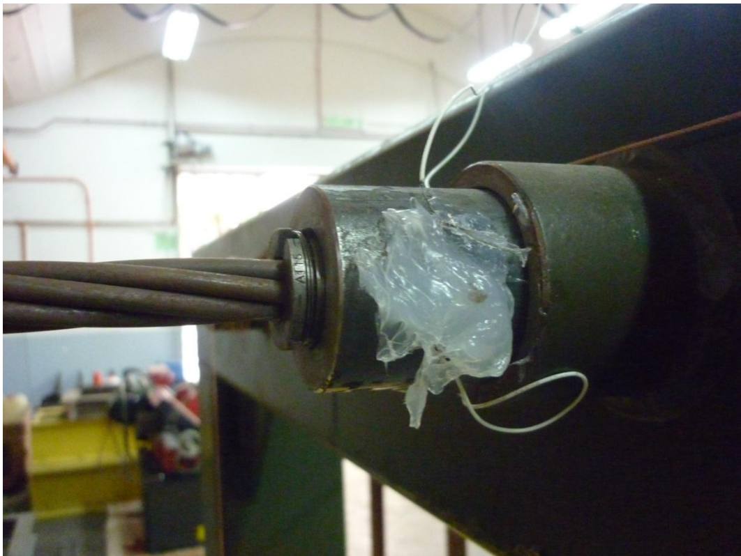
Figure 5.12: Strain gauge used on the wedge and barrel.
