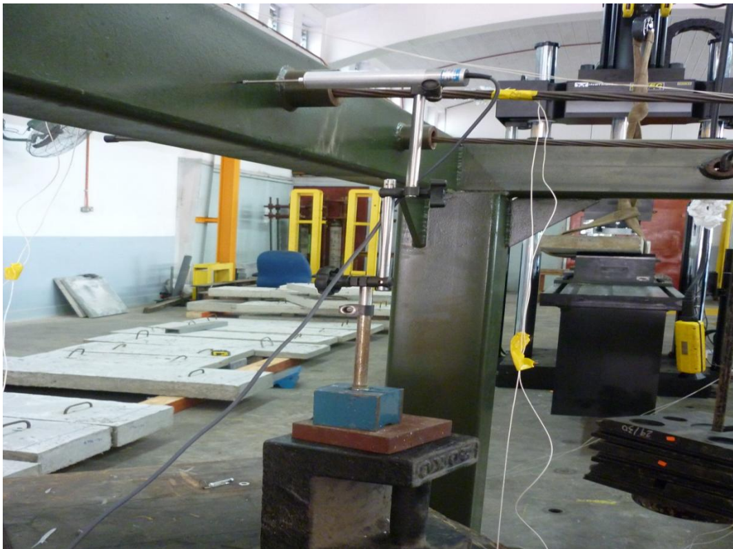
Figure 5.15: Linear variable differential transformer used on steel frame.
