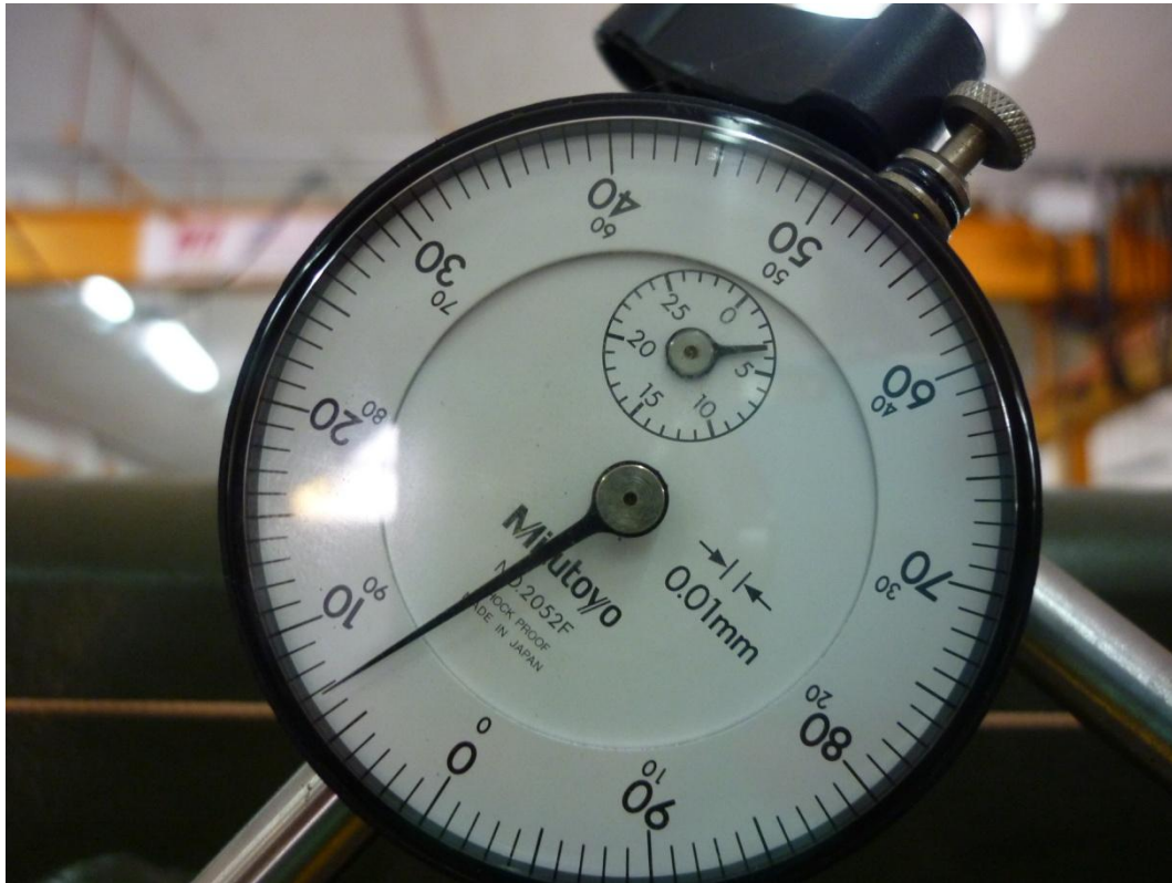
6 Figure 5.16: Dial indicator metric used on steel frame.
