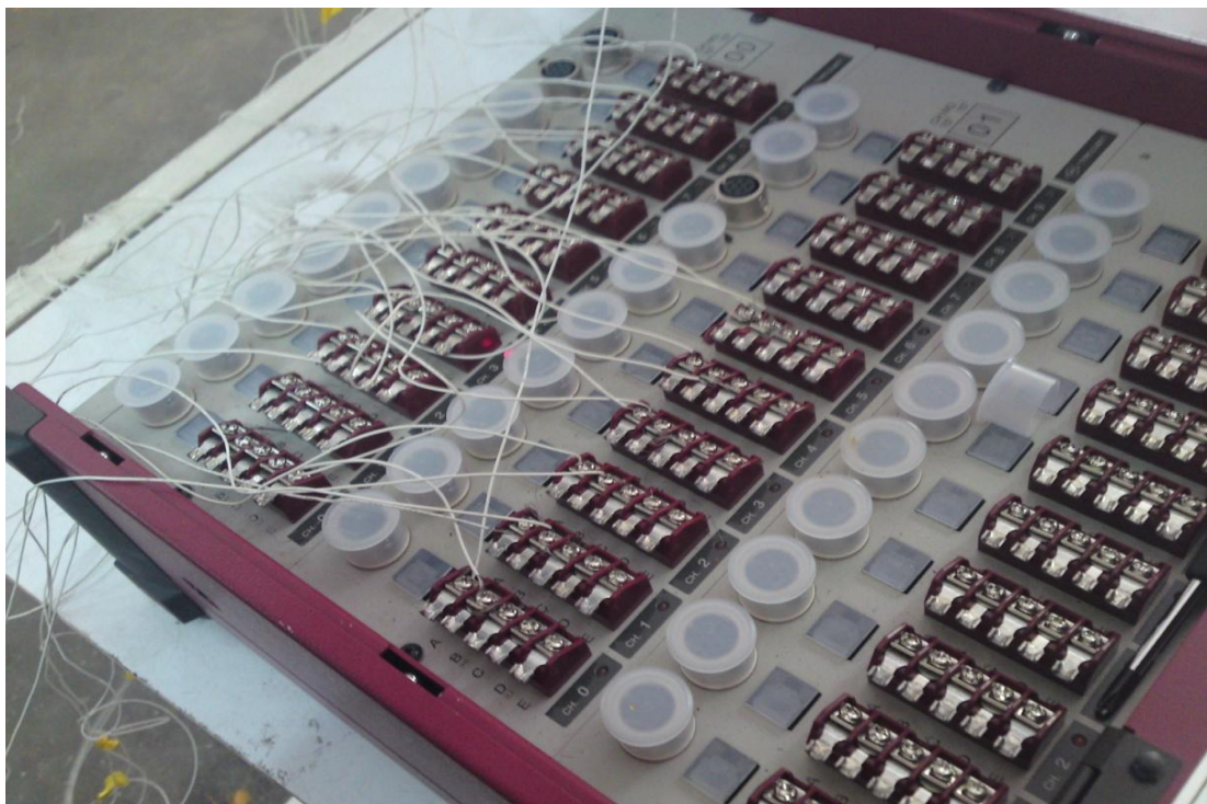
15 Figure 5.9: The channels of the TDS-530 data logger.
