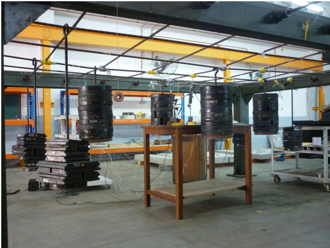
2 Figure 5.17: General view of the intensities and pattern of static loads.
