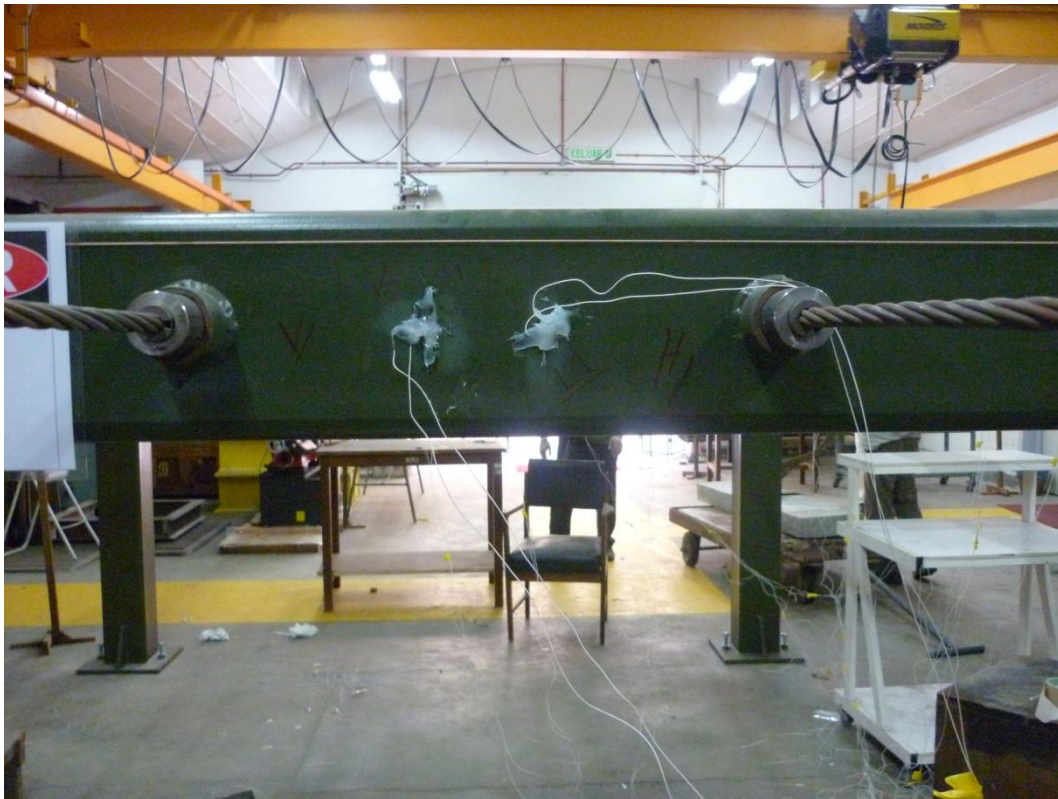
Figure 5.13: Strain gauge used on fabricated steel frame.
