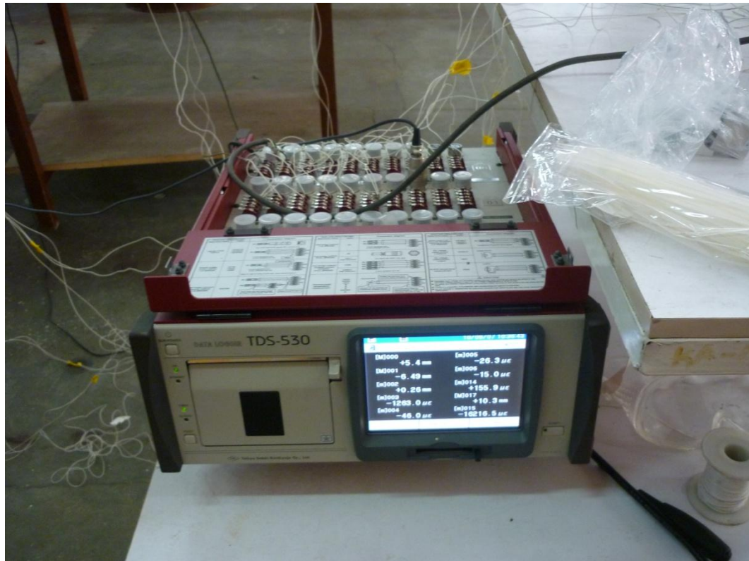
2 Figure 5.10: Top view of TDS – 530 Data logger.
