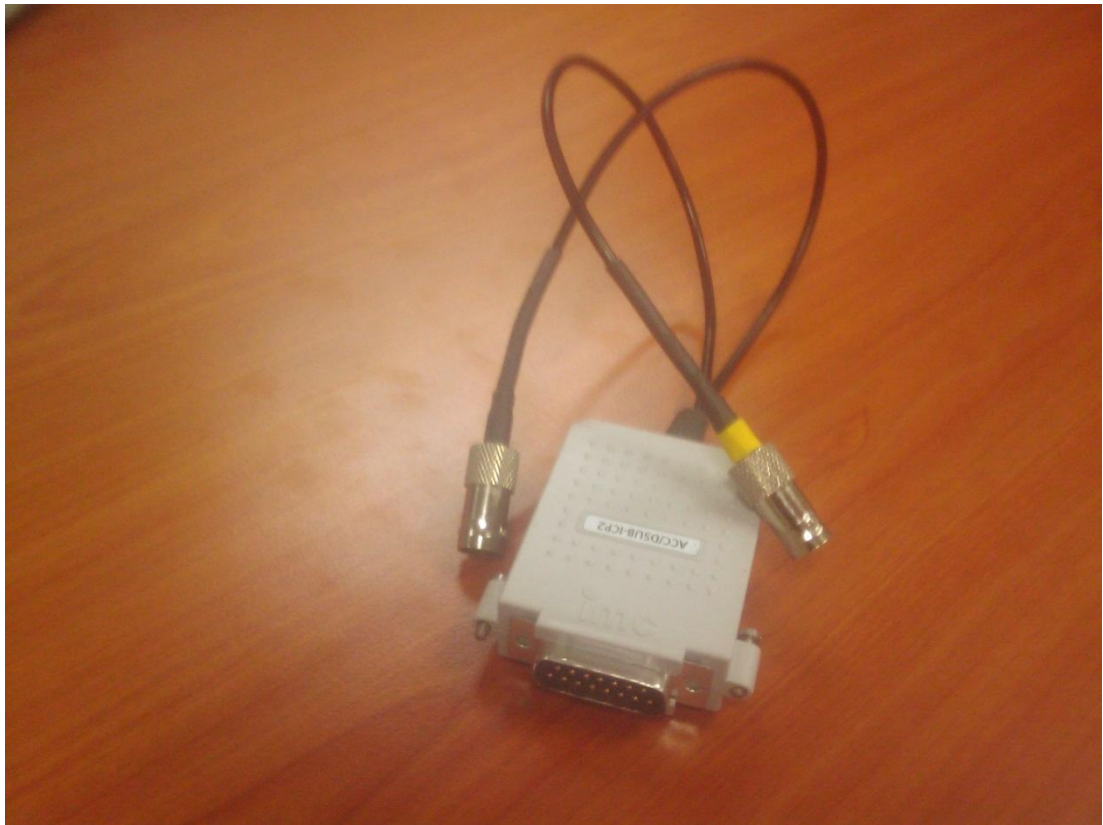
2 Figure 6.9: Top view of accelerometer-IMC connector device.
