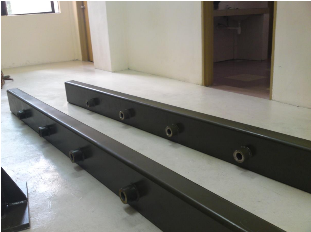
Figure 5.4: Steel beams fitted with hollow cylindrical steel sections.
