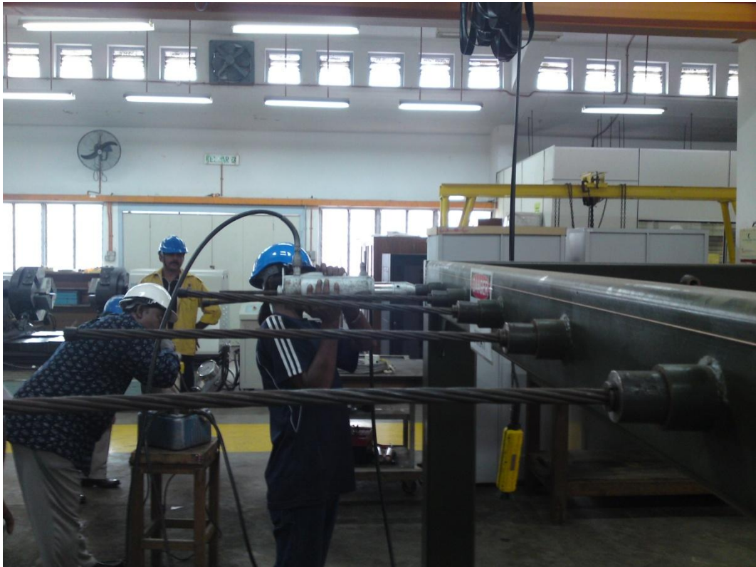
Figure 5.8: Tensioning of the cable with the pressure gauge.
