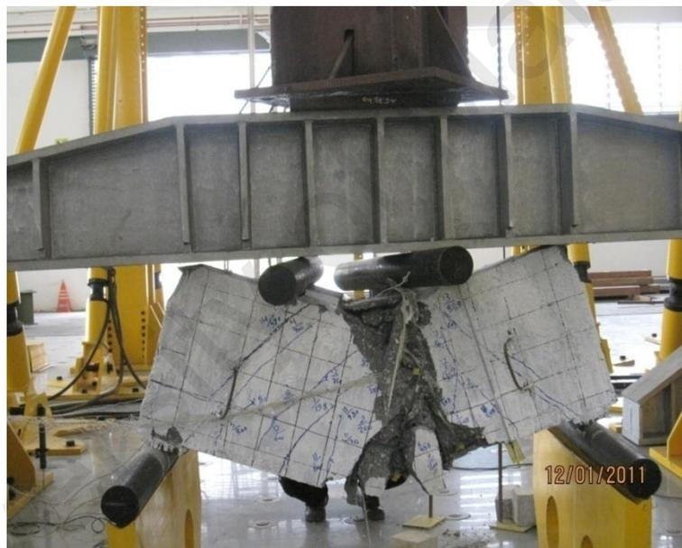
Figure 4.26: Failure of beam B7
