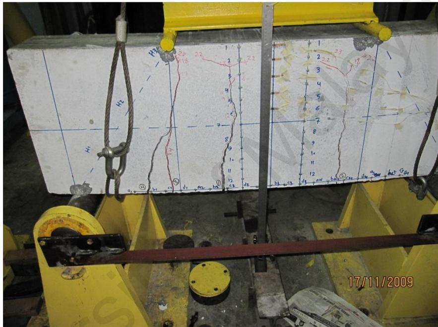
Figure 4.11: Crack progression in B1
