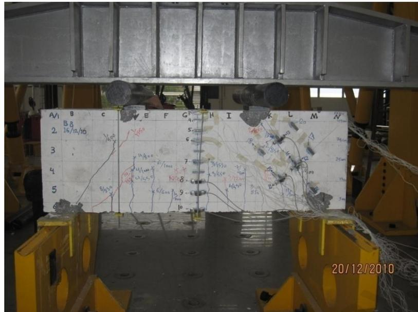
Figure 4.27: Failure of beam B8
