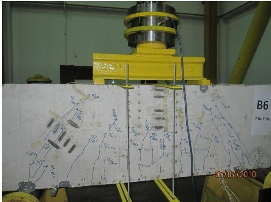
Figure 4.16: Crack progression in B6
