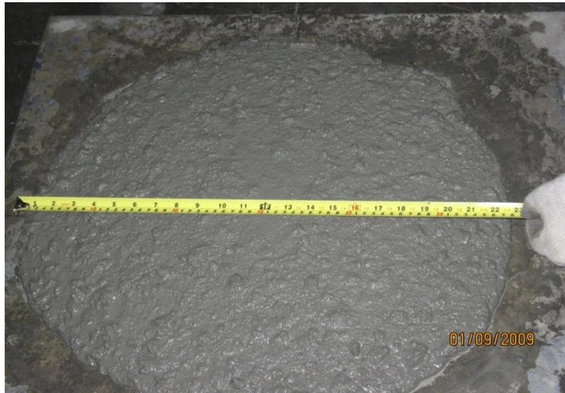
Figure 3.4: Workability slump value
