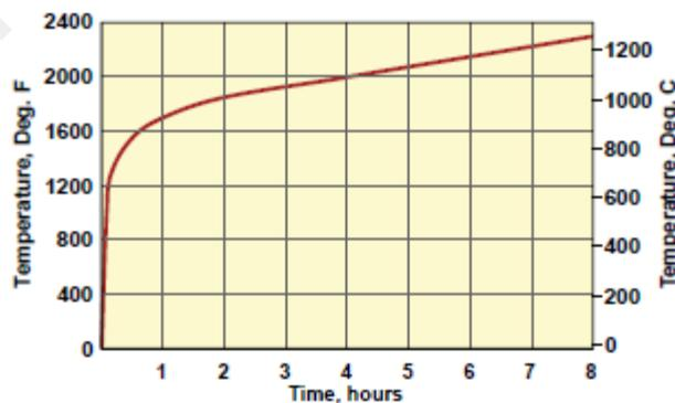
**Figure 2.12:** Time-Temperature Curve for ASTM Standard E-119
