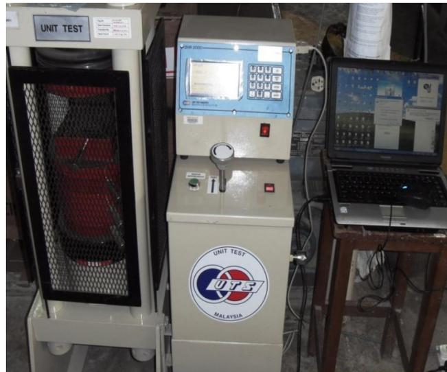
**Figure 3.7:** Wet and dry compressive strength apparatus
