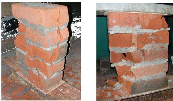
**Figure 2.13:** Masonry prism (Mohamad et al., 2005)
