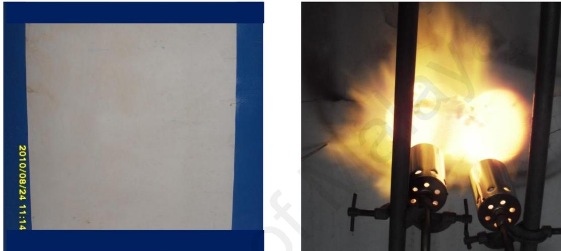
**Figure 3.13:** Flames for burning of CSPB masonry wall
