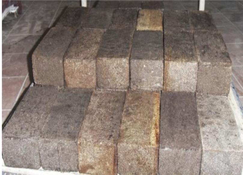
**Figure 3.8:** Compressed stabilised peat brick
