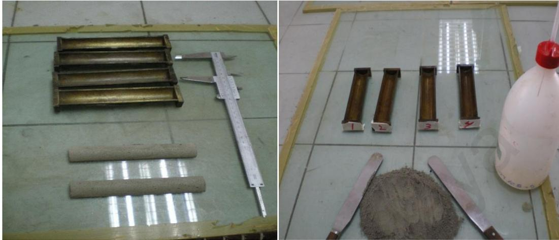
**Figure 3.5:** Apparatus of linear shrinkage
