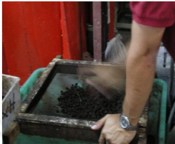
**Figure 3.2:** Dry peat soil being sieved through a 2 mm sieve
