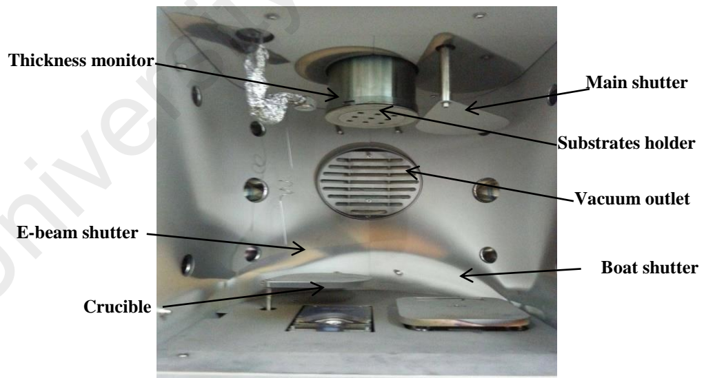
Figure 3.2: Picture of the inside chamber in the electron beam for the deposition process.
