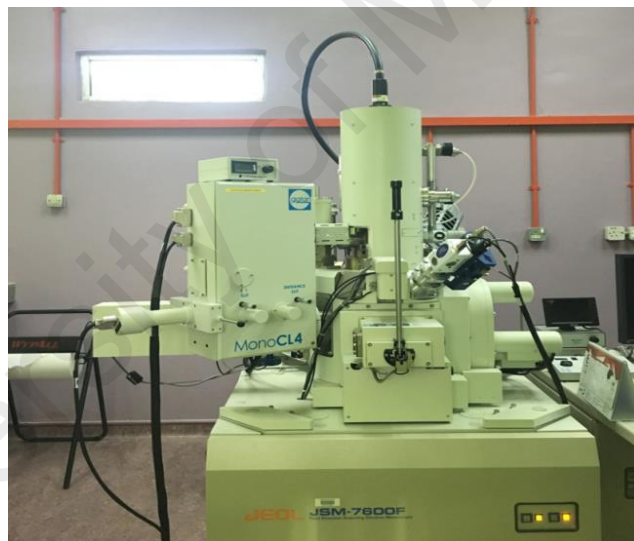
Figure 3.6: FESEM machine used in this work.
