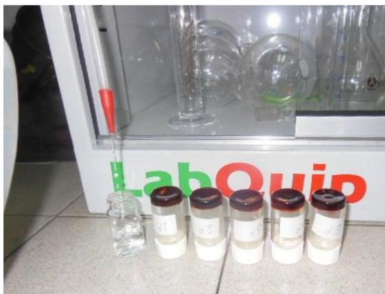
**Figure 3.2: Gel polymer electrolytes.**
