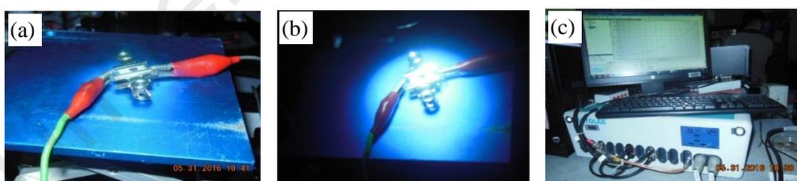
**Figure 3.7: Dye-sensitized solar cell (DSSC) (a) a complete DSSC, (b) DSSC under solar simulator light and (c) DSSC characterization by AutoLab station.**
