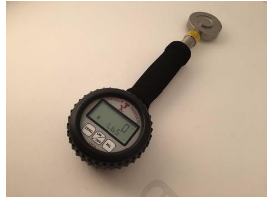
Figure 2-2 Welding Gun Pressure Gauge
