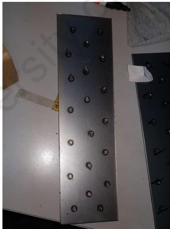
Figure 3-10 Test piece with spot welding
