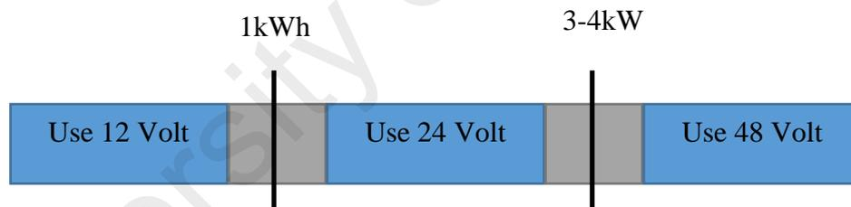
Figure 2.26 : Selection of the voltage level
