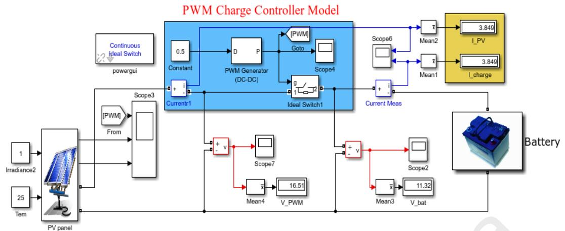
Figure 4.14: PWM Charge Control Model
