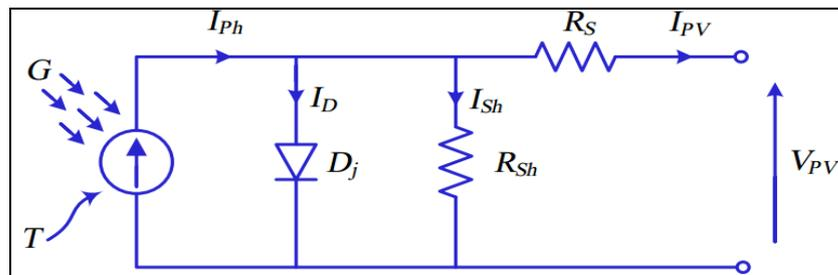
Figure 2.8: Complete general model of photovoltaic cell
