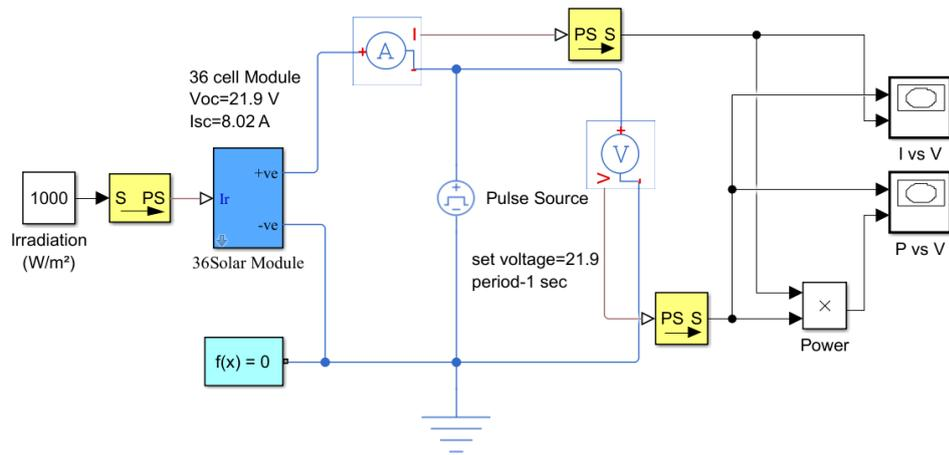
Figure 4.2: Model of Solar PV module to test output parameters
