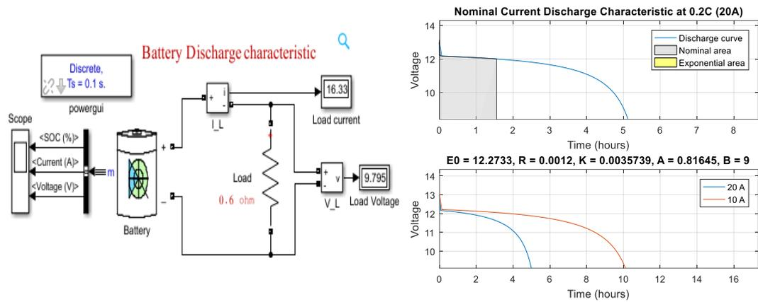
Figure 4.11: simulation discharge individual (VRLA) lead acid battery
