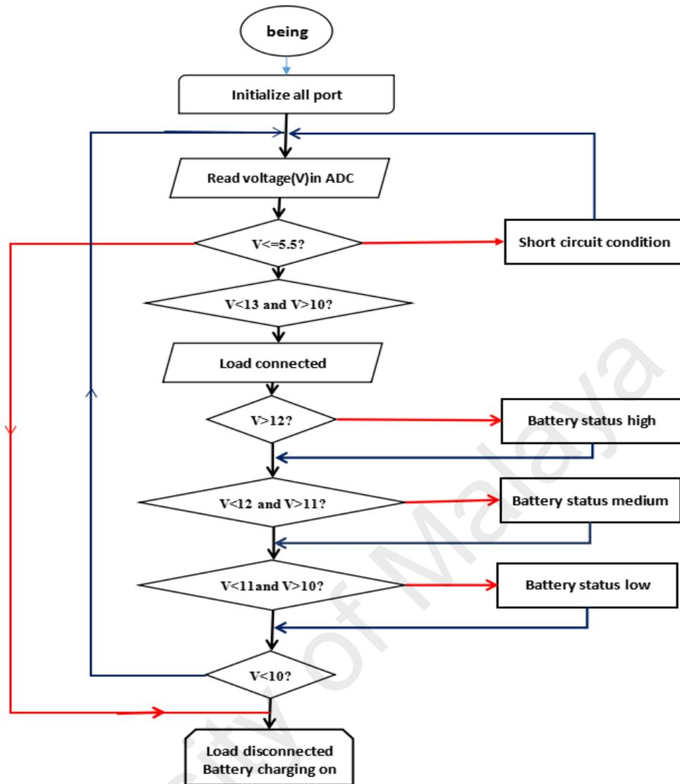
Figure 2.30: Flowchart of Charge Controller
