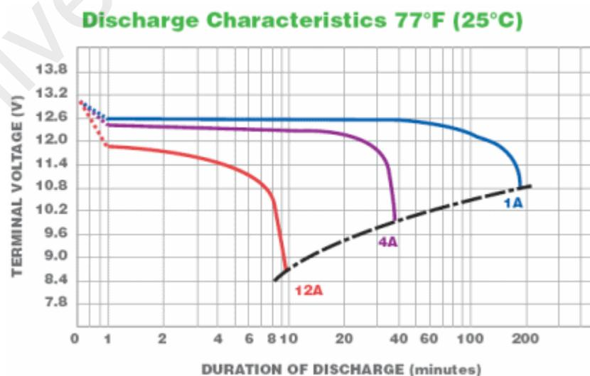
Figure 2.23: Discharge characteristics of the TR1.3-12V
