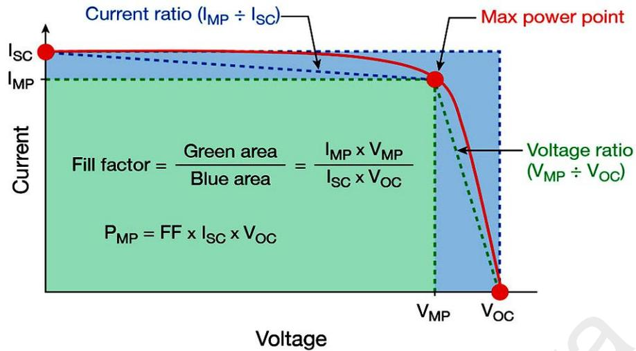
Figure 2.12: Photovoltaic module characteristics showing the fill factor
