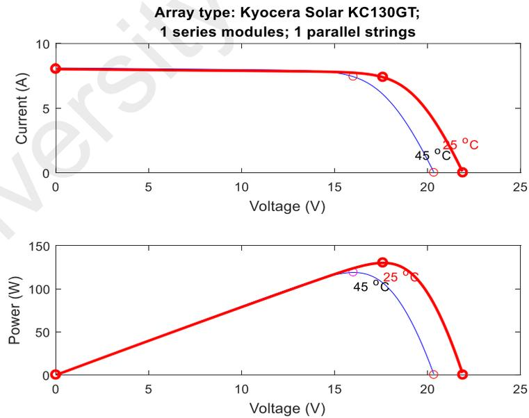
Figure 4.7: I-V&P-V properties at fixed irradiance with different temperature.
