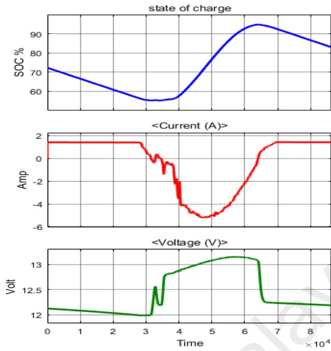
Figure 4.22: Case 1 simulation state of the battery during the sunny day
