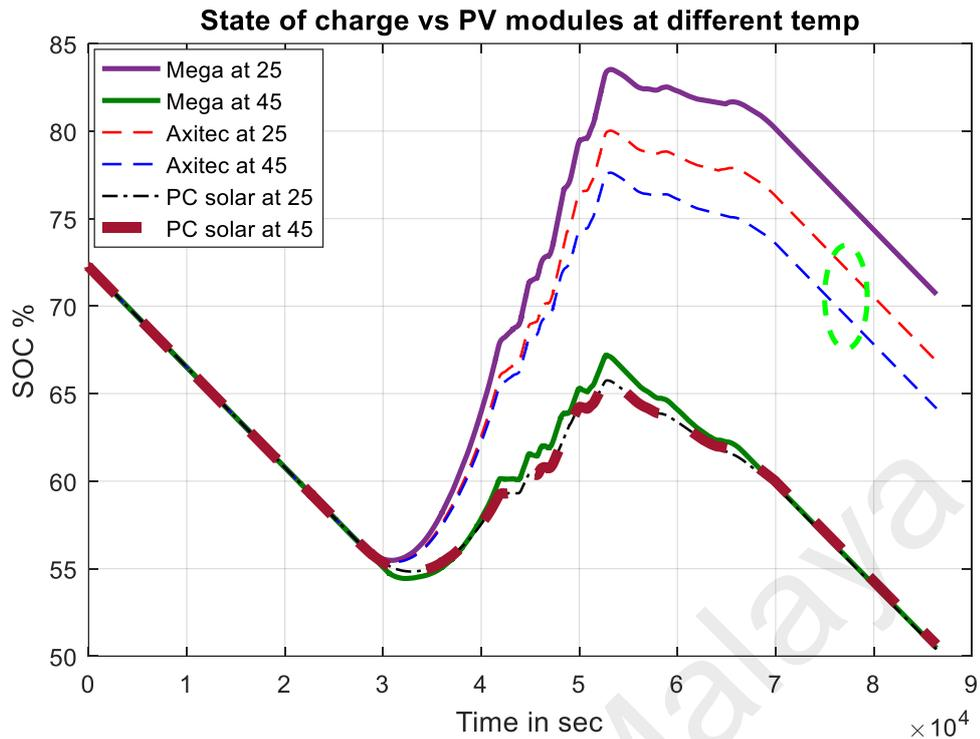
Figure 4. 28: State of charge vs. PV modules during a cloudy day
