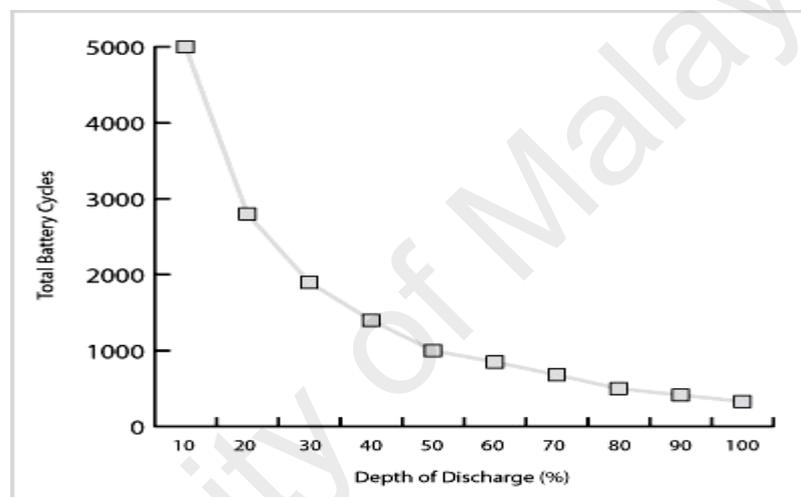
Figure 2.24 : Depth of Discharge vs Cycle Life
