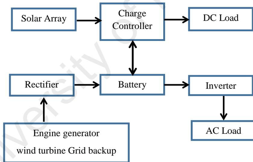
Figure 2.3: Diagram of the stand-alone PV hybrid system.
