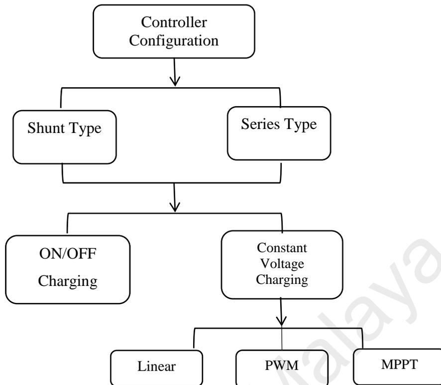
Figure 2.28 : Common Controller Typologies for Battery Charging
