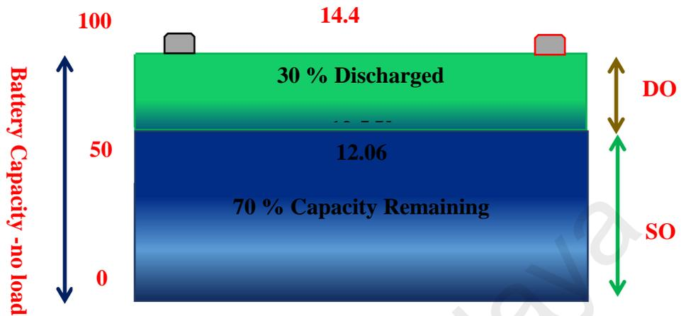
Figure 2.25 :SOC level of 12 V Battery
