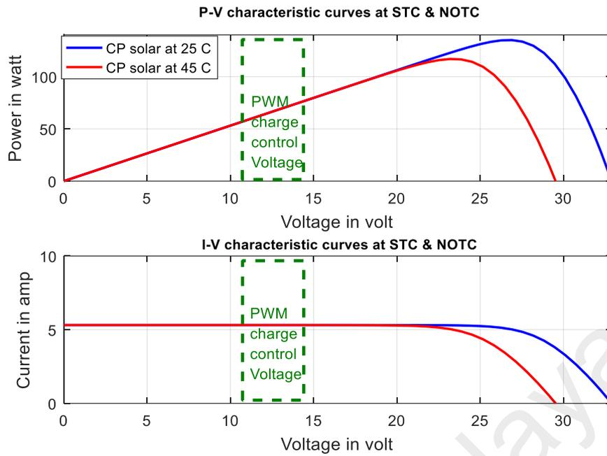
Figure 4.26: Photovoltaic module tested at a temperature
