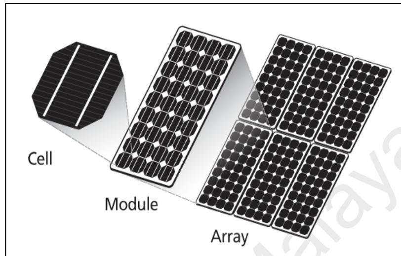
Figure 2. 6: Solar Module and solar PV Array
