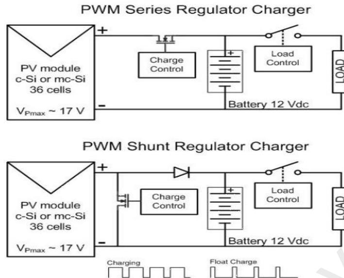
Figure 2.27: PWM series and shunt charger
