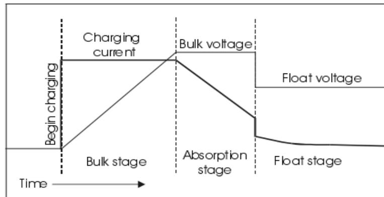
Figure 2.31: The diagram of charging stages of lead-acid battery
