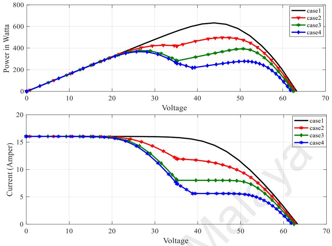
Figure 4.8 : I-V & P-V characteristic under partial shading condition
