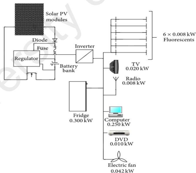
Figure 2.4: Typical of stand-alone PV System (Kanteh Sakiliba, Sani Hassan et al. 2015)
