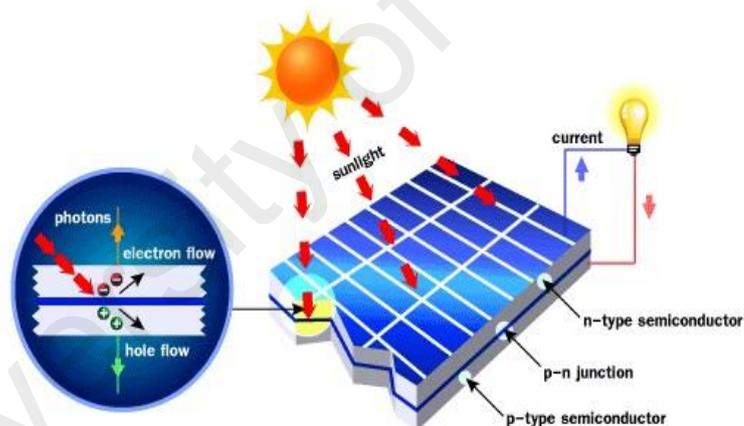
Figure 2.5: The Basic operating principle of a solar cell
