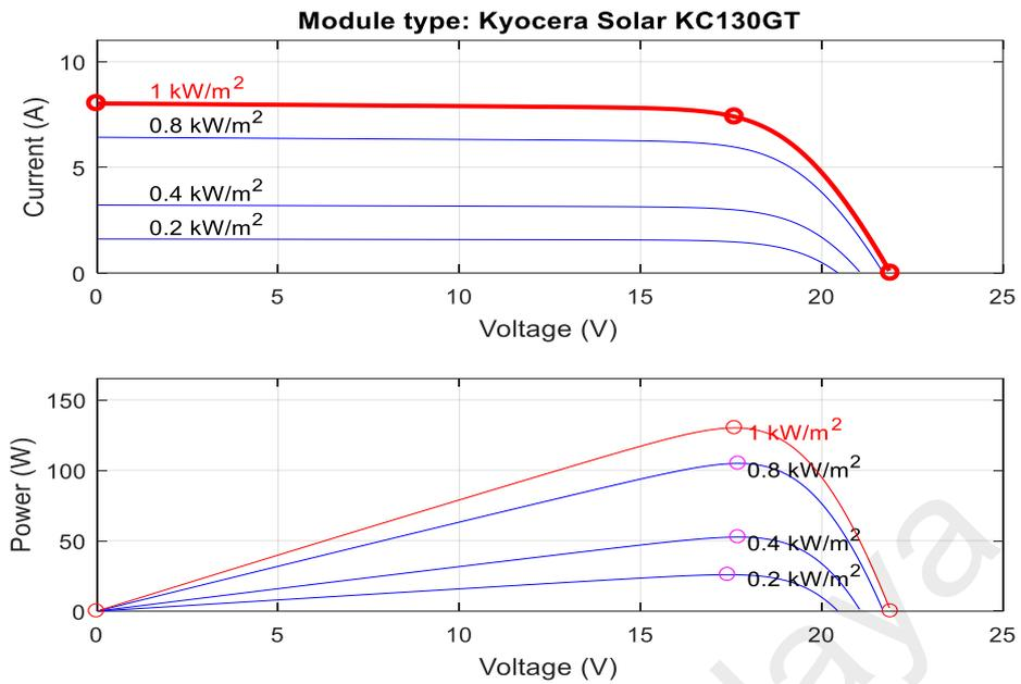
Figure 4.6: I-V&P-V properties at fixed temperature with varying irradiance.
