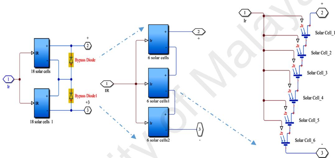
Figure 4.1: Model of solar cell module having 36 individual cells
