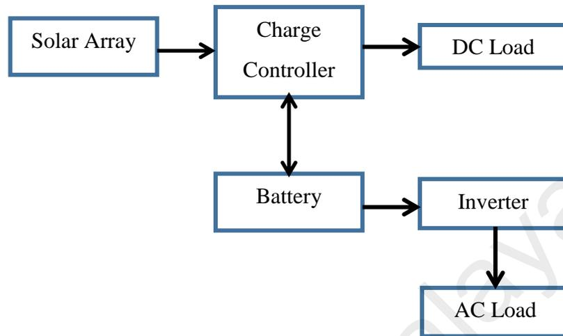
Figure 2. 2: Diagram of a stand-alone PV system with battery storage.
