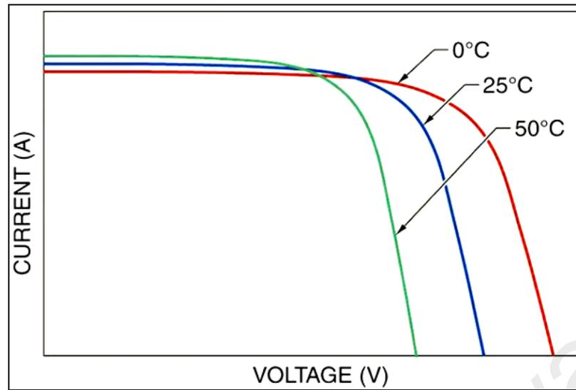
Figure 2.11: Voltage will drop due to temperature increase
