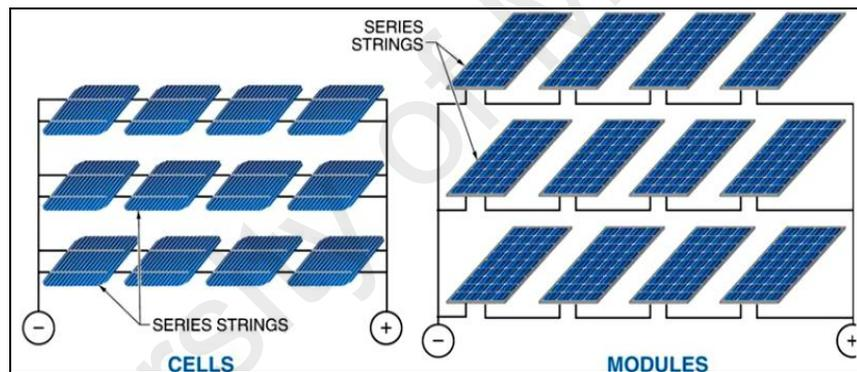
Figure 2.16 :Parallel connection PV module and array
