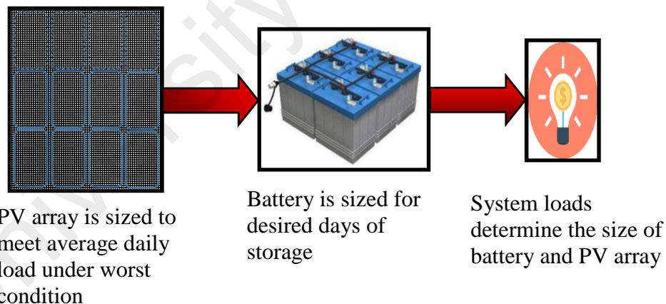
Figure 3.1: Selection and-sized components.
