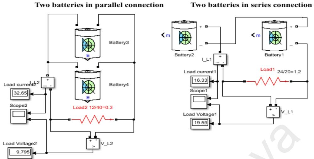
Figure 4.12: illustrated a combination batteries in Series / parallel connections
