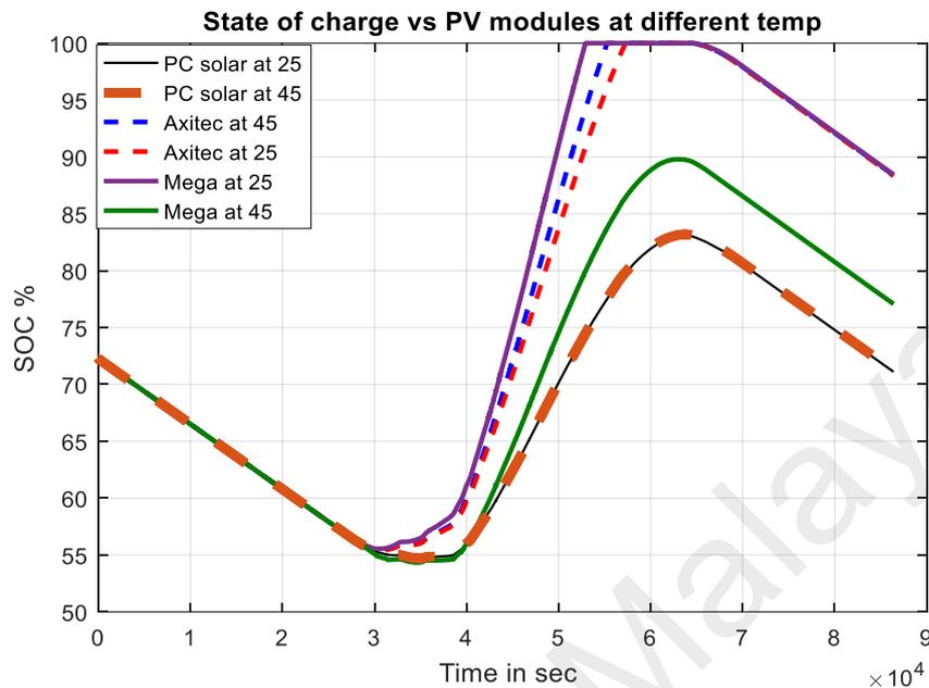
Figure 4.29: State of charge vs PV modules during sunny day
