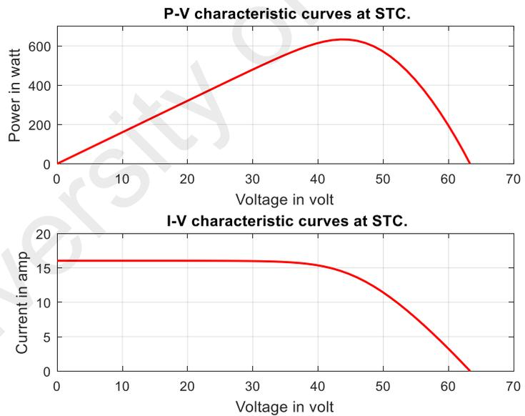
Figure 4.5: The I-V and P-V curve characteristics of PV array
