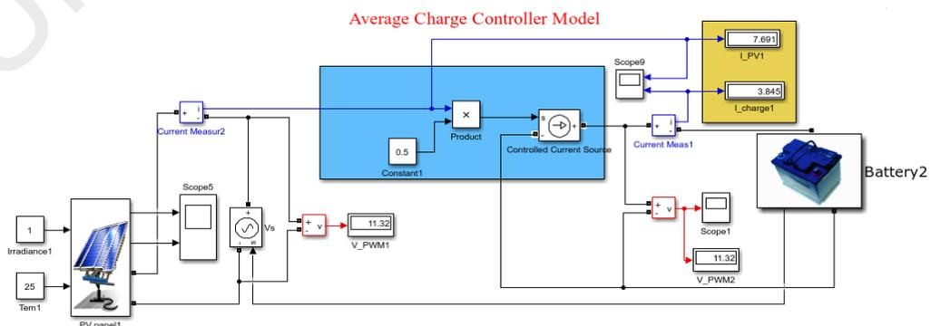
Figure 4.16: Average Charge Controller Model
