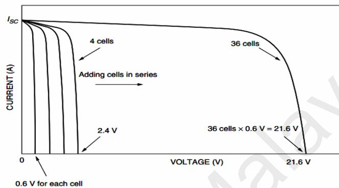
Figure 2.20: 36cells wired in series, parallel (Masters 2013)
