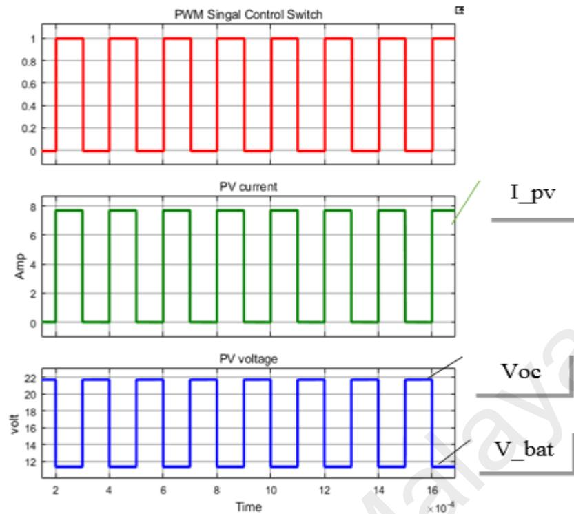
Figure 4.15: PV voltage and current, controlling by PWM signal
