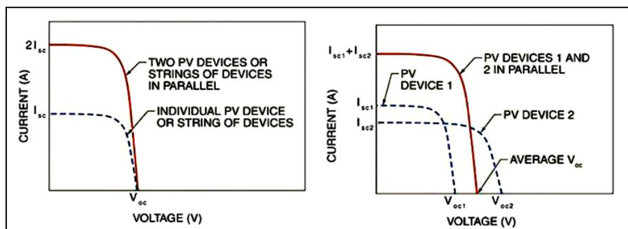
Figure 2.17: V-I outputs for similar module and dissimilar module
