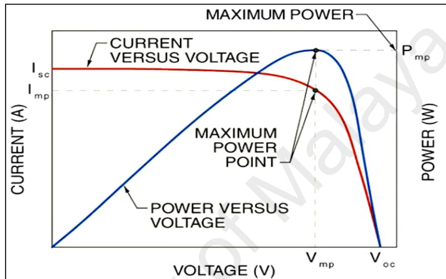
Figure 2.9: I-V properties of PV modules
