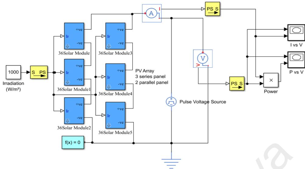
Figure 4.4: PV Array Model configuration
