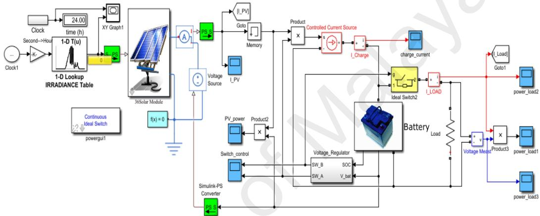
Figure 4.21: Simulink diagram DC load PV off-grid model
