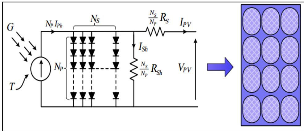
Figure 2.13: Solar model in parallel and series branches.
