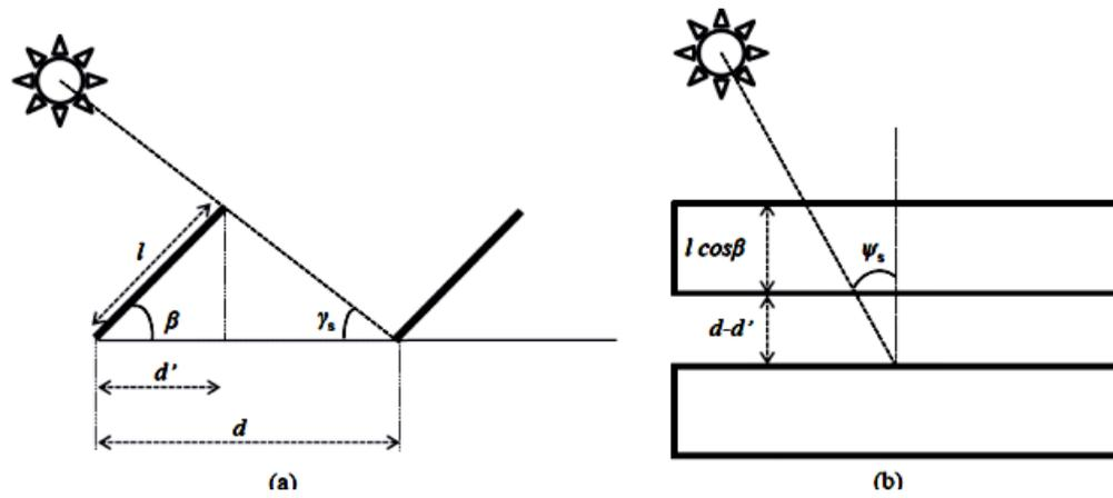
Figure 3. 6: The distance between panels (shadow length 'd-d')
