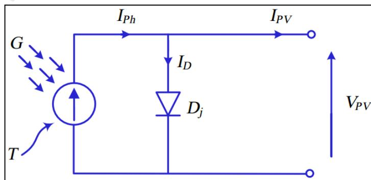
Figure 2.7: Simple model of photovoltaic cell
