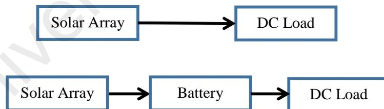
Figure 2. 1: Direct-coupled PV system.
