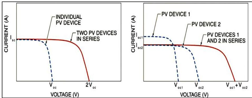
Figure 2.15: V-I outputs for similar module and dissimilar module
