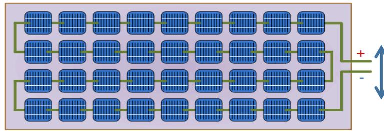
Figure 2.19: Typical 36 Cell Photovoltaic Panel
