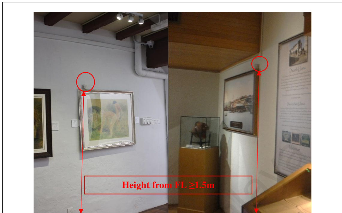
Figure 3.4: Placement of HOBO U12 External Data Logger at BPM (left) and PSM (right)
