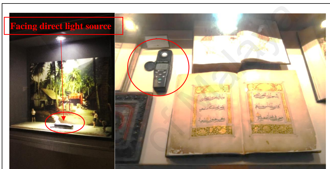
Figure 3.6: Placement of TENMARS Light Meter inside the display's showcase cabinet at MIPIM (left) and PSM (right)
