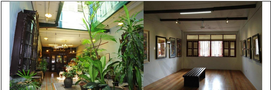
Figure 5.10: The uses of internal courtyard, ceiling fans and window openings for ventilation purposes at SYSM (left) and BPM (right)
