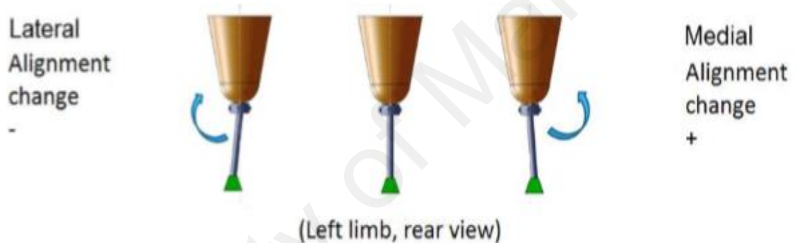
Figure 3.6: Foot and socket shifting in frontal aspect (Chen, 2012)
