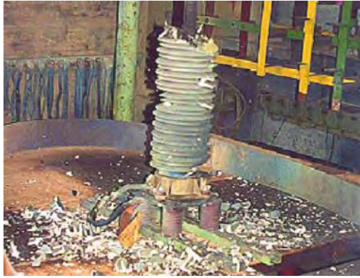
Figure 2.7: Short circuit test (a) Porcelain and (b) Polymer (Steinfeld K., Gohler R., & D, 2003)
