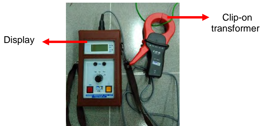
Figure 3.8: Experimental set up for leakage current measurement using SCAR10
