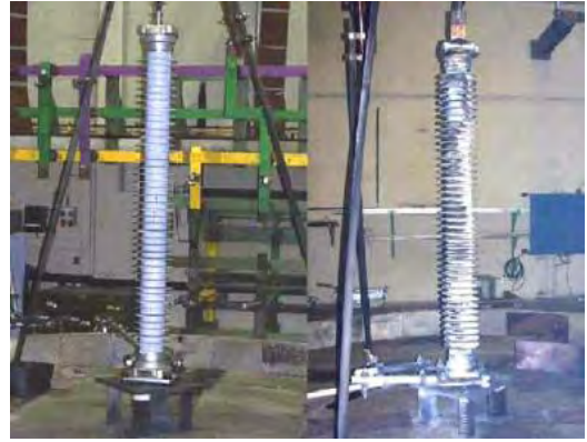
Figure 2.7: Short circuit test (a) Porcelain and (b) Polymer (Steinfeld K., Gohler R., & D, 2003)
