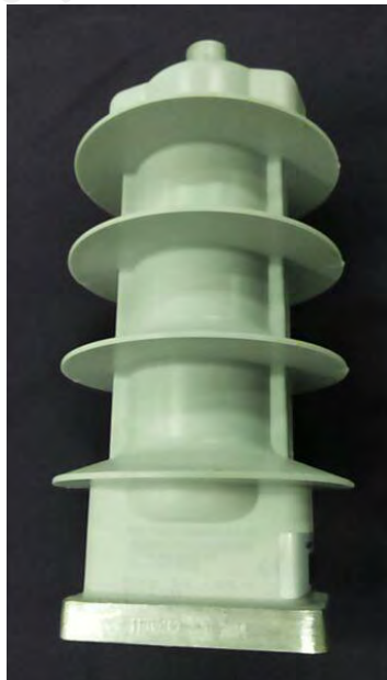
Figure 3.1: 11kV zinc oxide surge arrester with silicone rubber housing
