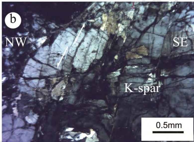
**Figure 4.10:** Microstructures from Bukit Perak granite (Location: Bina Quarry) indicating dextral shearing: a) shear band and oblique foliation; b) antithetic fracture in K-feldspar. Movement of fracture (sinistral) is opposite of the sense of shear in mylonite. All images under crossed nicol. Refer to Figure 4.4 for location of samples.
