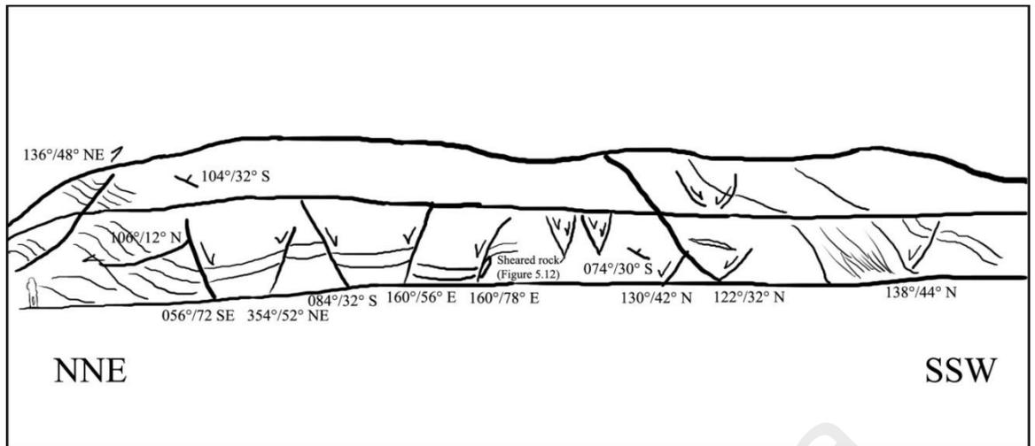
**Figure 5.11:** Sketch of D1 and D3 faults set, showing both reverse and normal movement. Location: Kuala Ketil. Geologist (lower left) is 1.6 m in height.
