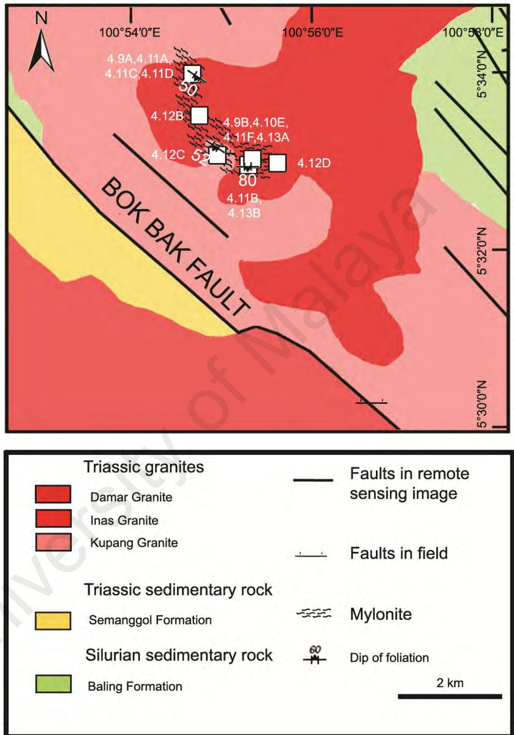
**Figure 4.6:** Mapped shear zone in Baling-Gerik granite. Location of figures for samples is indicated by squares. Division of granitic bodies based on Burton (1972).
