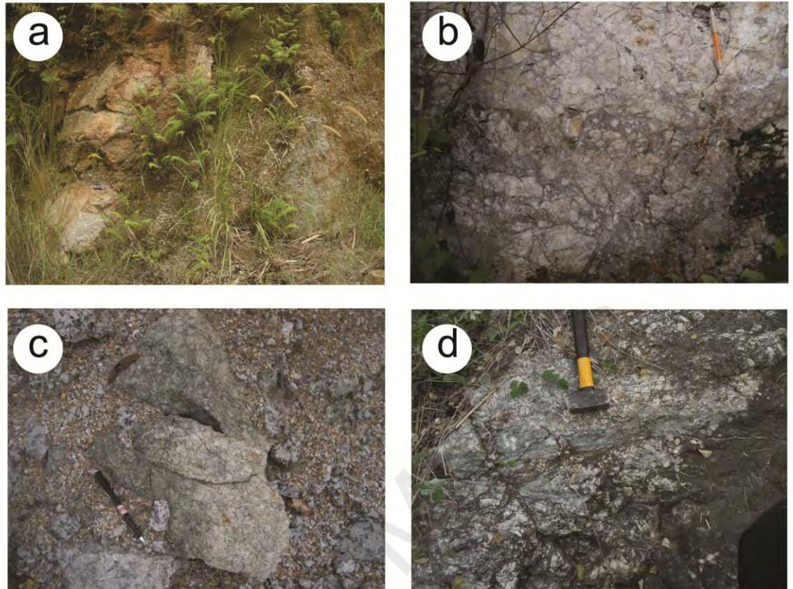
**Figure 5.2:** Brittle fault rocks in Bok Bak Fault: a) Fault breccia in Bukit Perak Granite (Location: Pati Quarry); b) – c) Cataclasite in granite (Location: b) Lubok Merbau; c) TAHB Quarry; d) Brittle shear band in Bintang Hills Granite (Location: Baling-Gerik Highway). a) – c) Pencil as scale; d) Hammer as scale. For locations refer to Figure 2.7.
