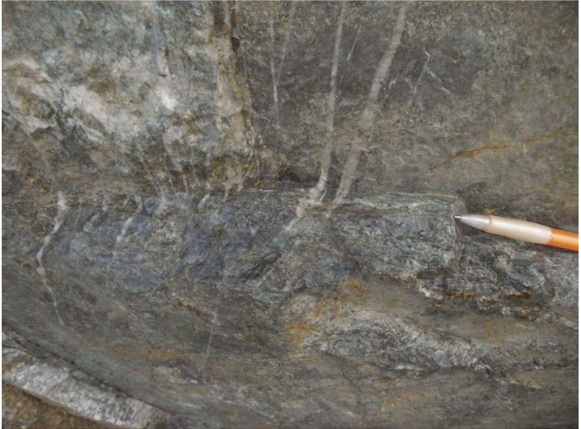
**Figure 4.5:** En echelon quartz filled fracture of Bukit Perak granite. View is looking towards NE. Location: Bina Quarry. Pencil as scale.
