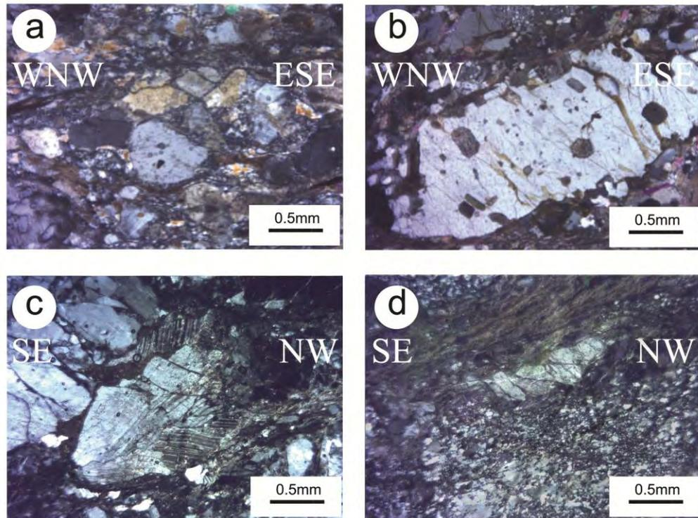
**Figure 4.13:** Microstructure showing deformation of feldspar: a) K-feldspar with both ductile (recrystallization of fine grains at feldspar rim) and brittle (fracturing) deformation); b) – c) Feldspar porphyroclast cut by fractures. Note twinning c); d) K-feldspar showing ‘bookshelf’ fracturing. Samples locations: a) – b): K173, Baling-Gerik Highway; c) – d) Bina Quarry. All images under crossed nicol. Refer to Figure 4.4 & 4.6 for location of samples.
