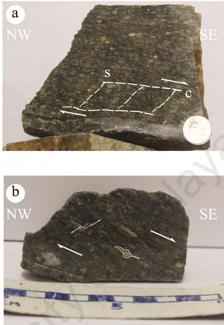
**Figure 4.9:** Oriented hand specimens of mylonite showing kinematic indicators: a) S-C structures; b) Mantled feldspar porphyroclast, and antithetic (sinistral) shearing in feldspar clast. Samples are cut parallel to stretching lineations. Samples location: K173, Baling-Gerik Highway. Coin as scale for a). Refer to Figure 4.6 for location of samples.
