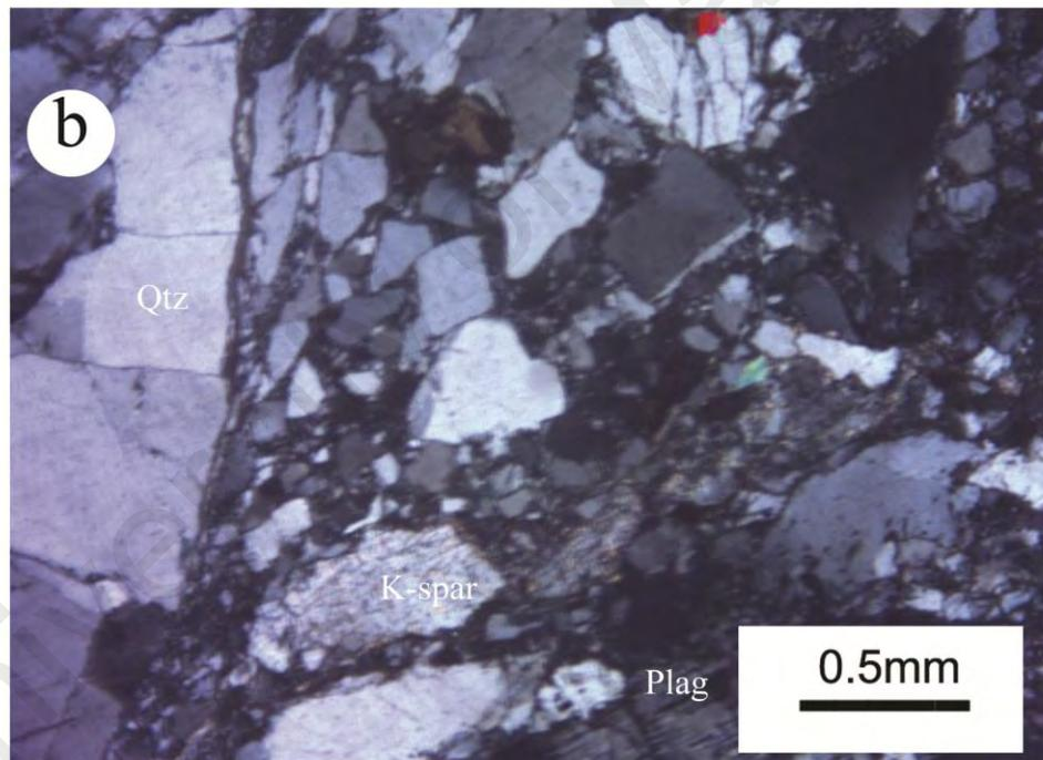
**Figure 5.13:** Photomicrograph of cataclasite formed in granite: a) Bukit Enggang Granite (Location: Sankojaya Quarry); b) Bintang Hills Granite (Location: Baling-Gerik highway). Images under crossed nicol. For locations refer to Figure 2.7.
