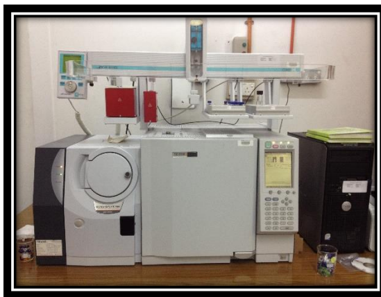
Figure 2.4: Hewlett Packard HP 6890 series mass selective detector linked to a GCMS-QP 2010 Plus Shimadzu gas chromatograph.
