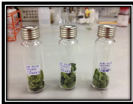
Figure 2.3: Leaves sealed in 20 mL capped vials ready for HS-SPME.
