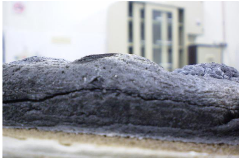
Figure 2.1: Intumescent coating after the Bunsen burner test (Yew & Ramli Sulong, 2012)
