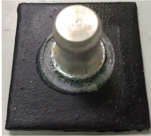
Figure 3.11: The dolly was adhered to the coating using epoxy glue
