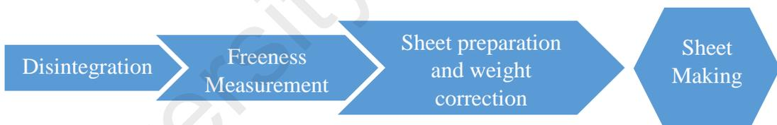
**Figure 3. 3** Flowchart of sheet making process
