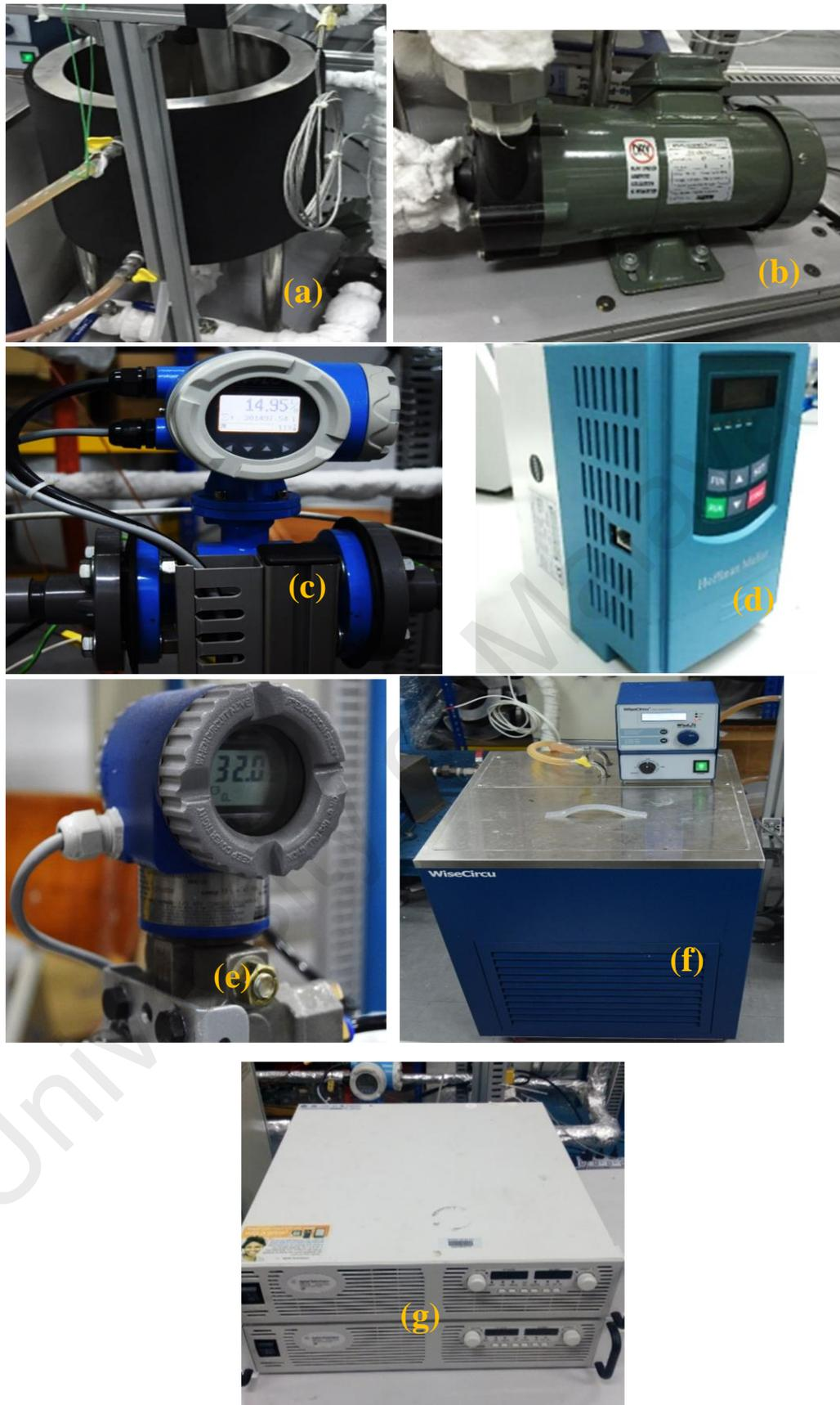
**Figure 3. 7** Photographs of equipment's (a) Stock tank, (b) Magnetic gear pump, (c) Magnetic Flow meter, (d) Hoffman Muller inverter, (e) Differential Pressure Transducer, (f) Cooling unit, (g) Power supply.
