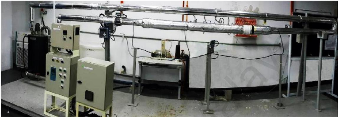
**Figure 3. 2** photograph of the experimental setup of suspensions flow.
