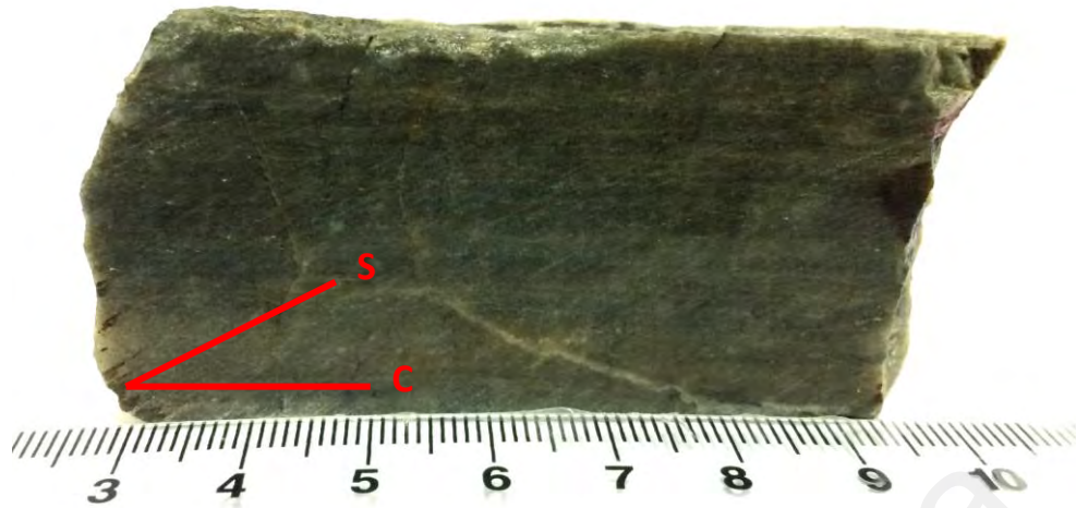
Plate 3.8: A sample of mesomylonite from BTFZ. The grain size is finer than the protomylonite and it has higher matrix content (50-90%). The C-surfaces are more distinct than the faint S-surfaces.
