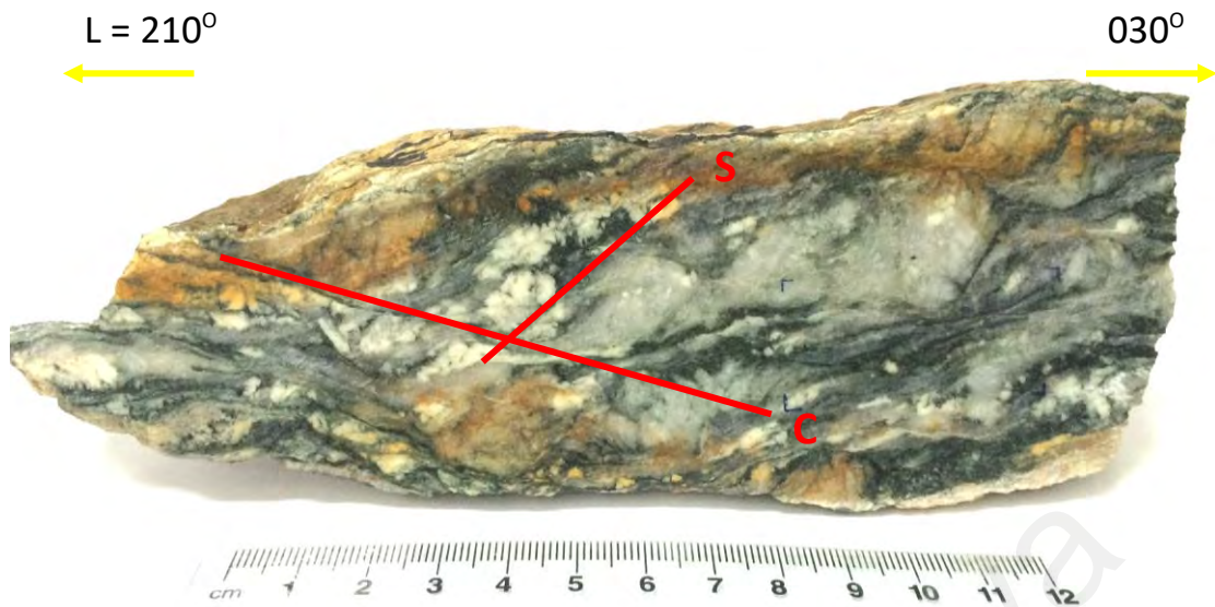
Plate 3.6: A sample of protomylonite from BTFZ. The preferred orientation of tabular to ellipsoidal feldspar porphyroclasts is parallel to S-surfaces. The elongated quartz aggregates and mica strings are mainly aligned parallel to S-surfaces but some are aligned along the C-surfaces.
