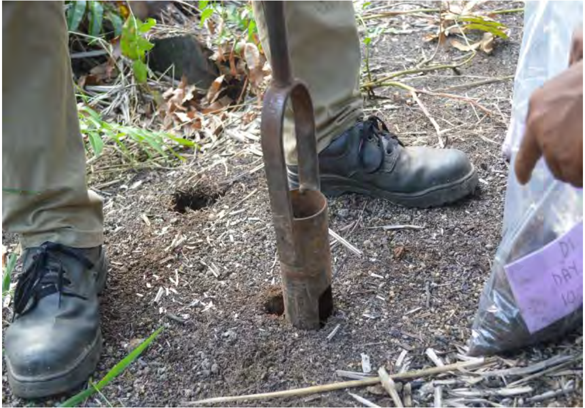
Figure 4.7: Collections of 5 different depths soil sample using auger
