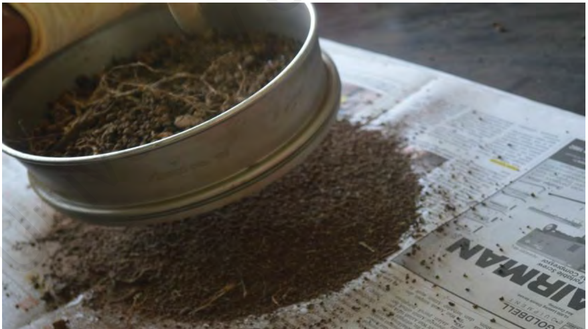
Figure 4.8: Sieving of soil samples
