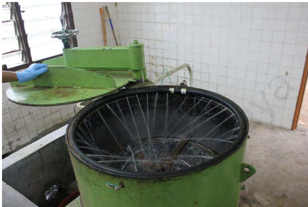
Figure 4.11: Separation using depalper machine
