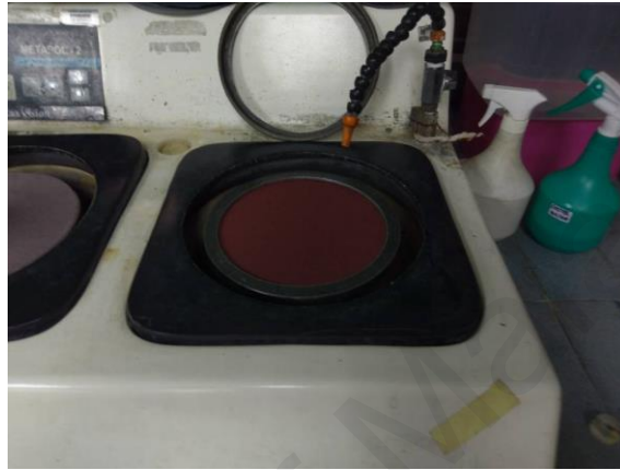
Figure 3.8: Grinding and polishing machine.
