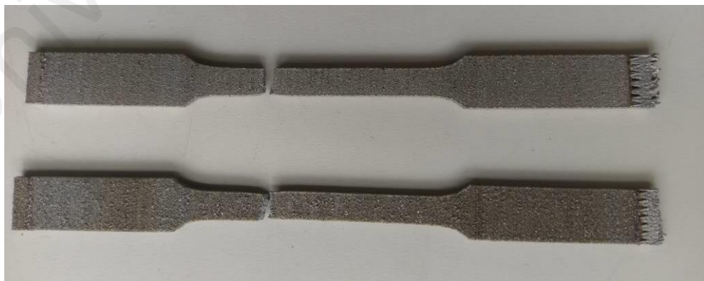
Figure 4.6: samples after break due to the tensile test
