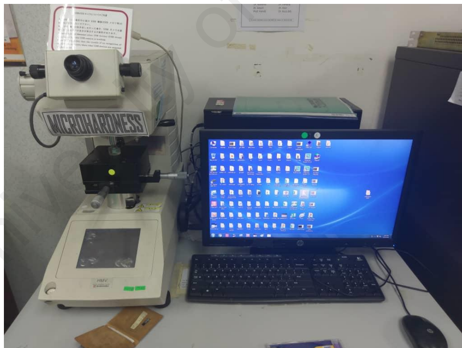
Figure 3.11: Micro hardness equipment used in this study.
