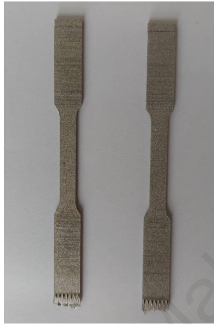
Figure 3.2: 316L stainless steel samples used in this project
