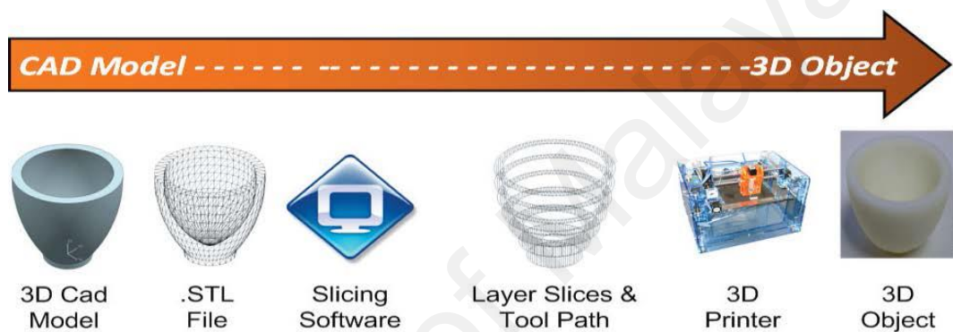
Figure 2.2: the sequence of AM processes starting from 3D model and finishing to manufactured part
