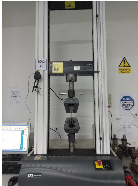
Figure 3.4: Instron tensile test equipment
