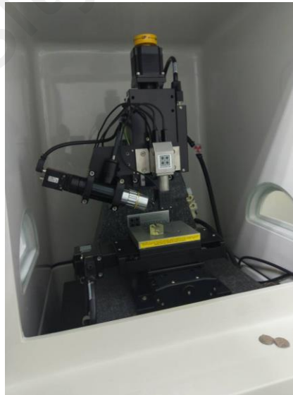
Figure 3.10: Sample placed in the chamber for nanoindentation test.
