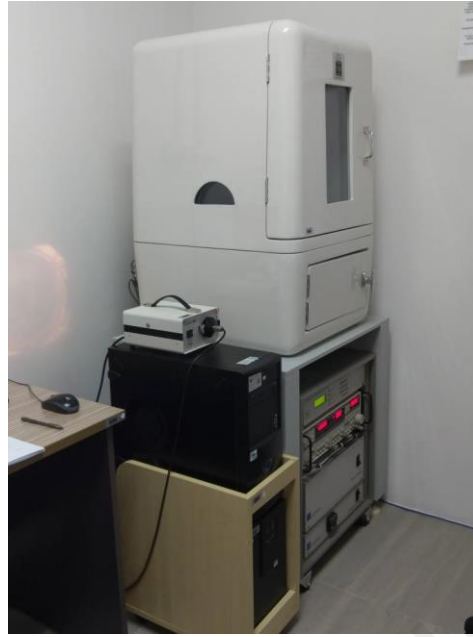
Figure 3.9: Nanoindentation equipment available at UM.
