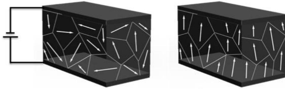
Figure 2. 9 Process of polarization and polarization surviving (Caliò, 2013)
