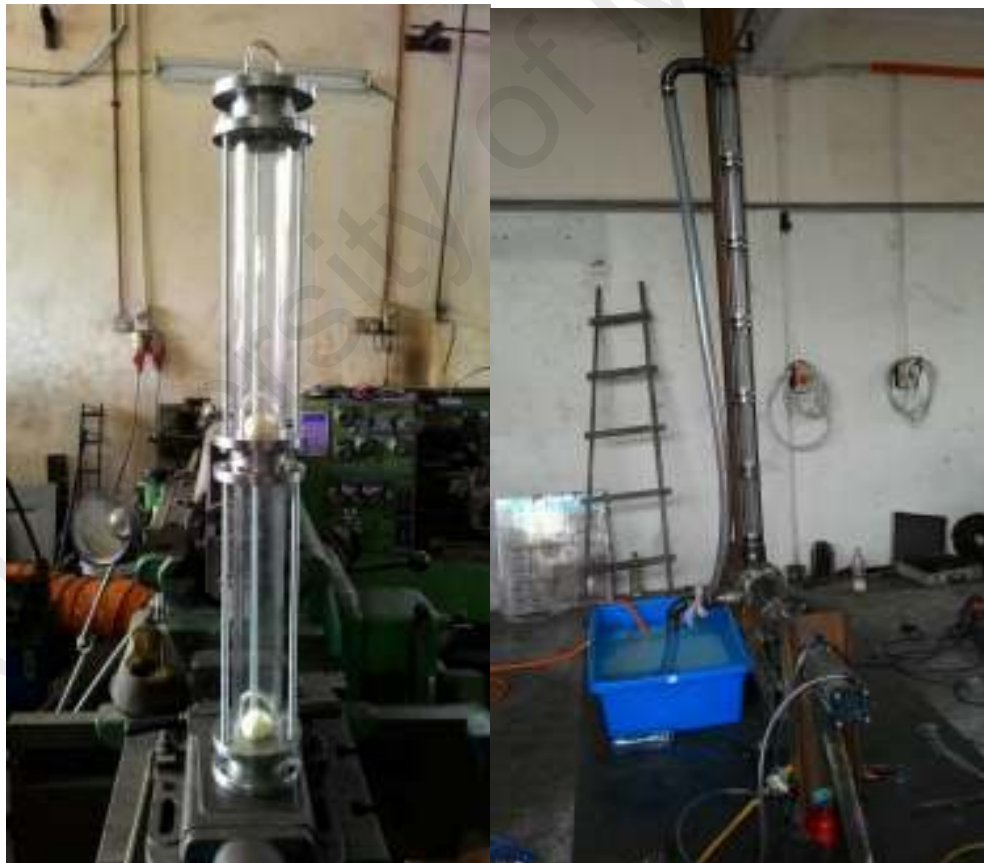
Figure 3.4: One way ball valve inside cylinder
