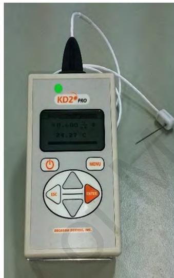
**Figure 3.1:** Photograph of the thermal properties analyzer (KD2 pro).
