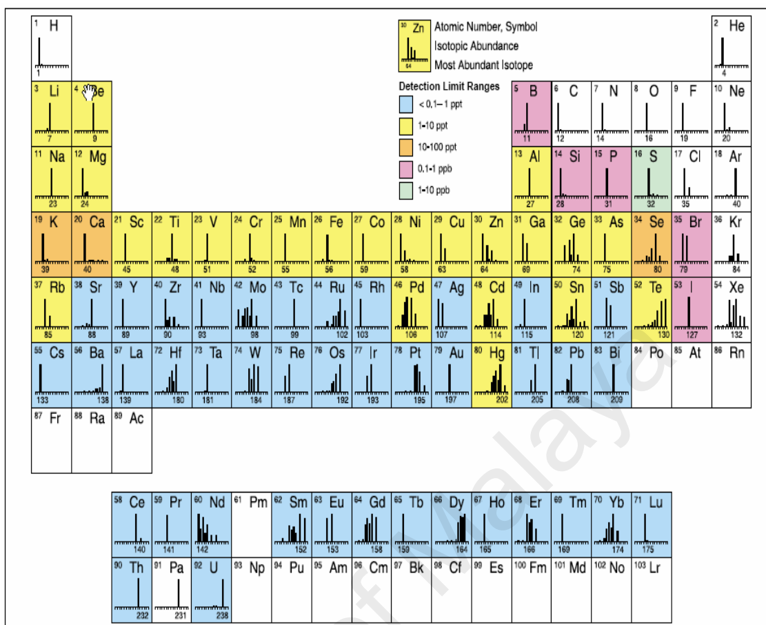
Figure 3.14: Representation of ICP-MS Technical Specifications in a Periodic Table
