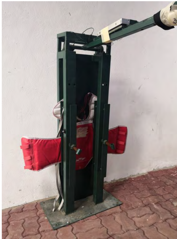
Figure 3.3: Placement of electronic body protector on the mechanical pendulum
