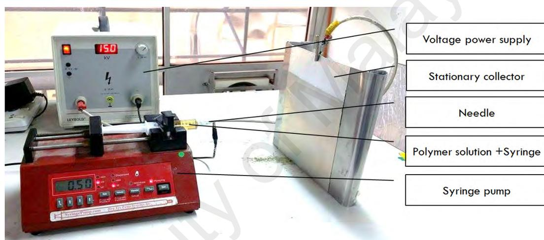
Figure 3.2: An electrospinning setup.
