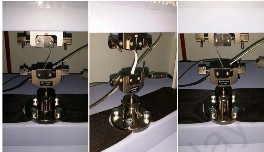
Figure 4.12: Buckling of specimens at the end of cyclic-relaxation tests.
