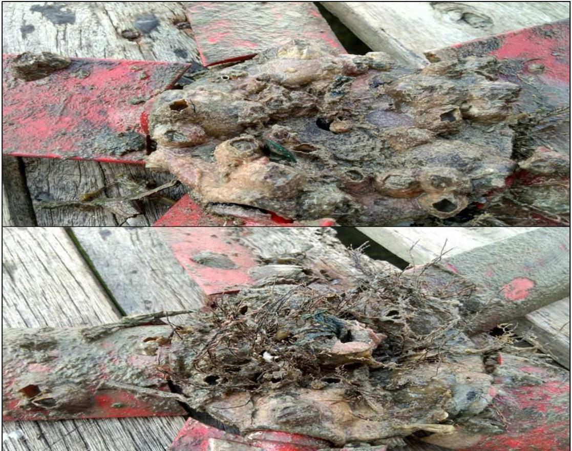
**Figure 4.33:** Hub area of coated dummy, up (front), down (back).
