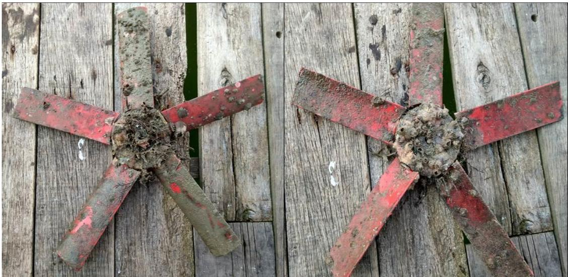
**Figure 4.31:** Coated dummy turbine after the marine bio-fouling test, left (front), right (back).
