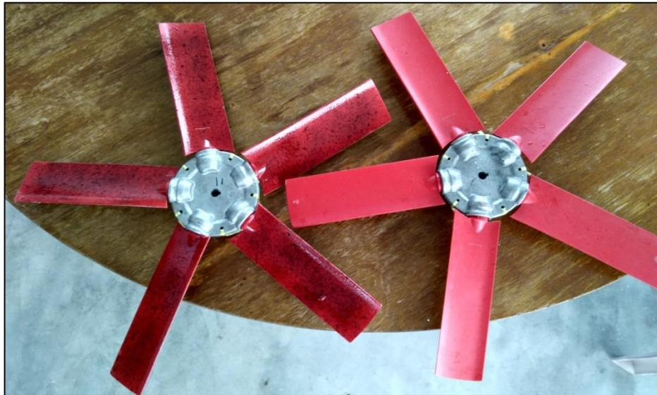
**Figure 4.29:** Dummies turbine before the marine bio-fouling test, left (coated), right (uncoated).
