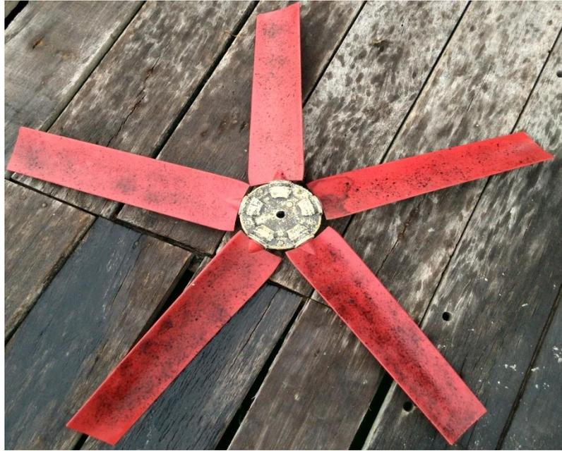
**Figure 3.2:** Five-bladed turbine used for the field test.
