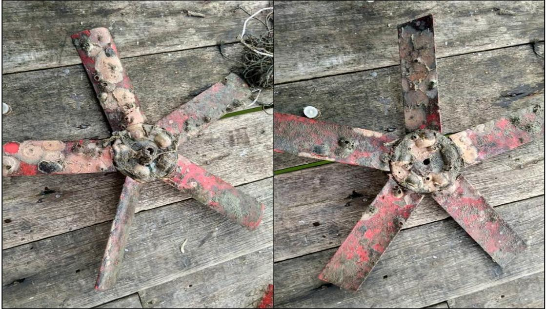
**Figure 4.32:** Uncoated dummy turbine after the marine bio-fouling test, left (front), right (back).
