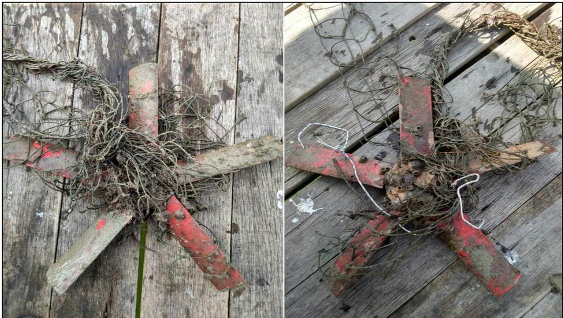
**Figure 4.30:** Dummies turbine after the the marine bio-fouling test, left (coated), right (uncoated).
