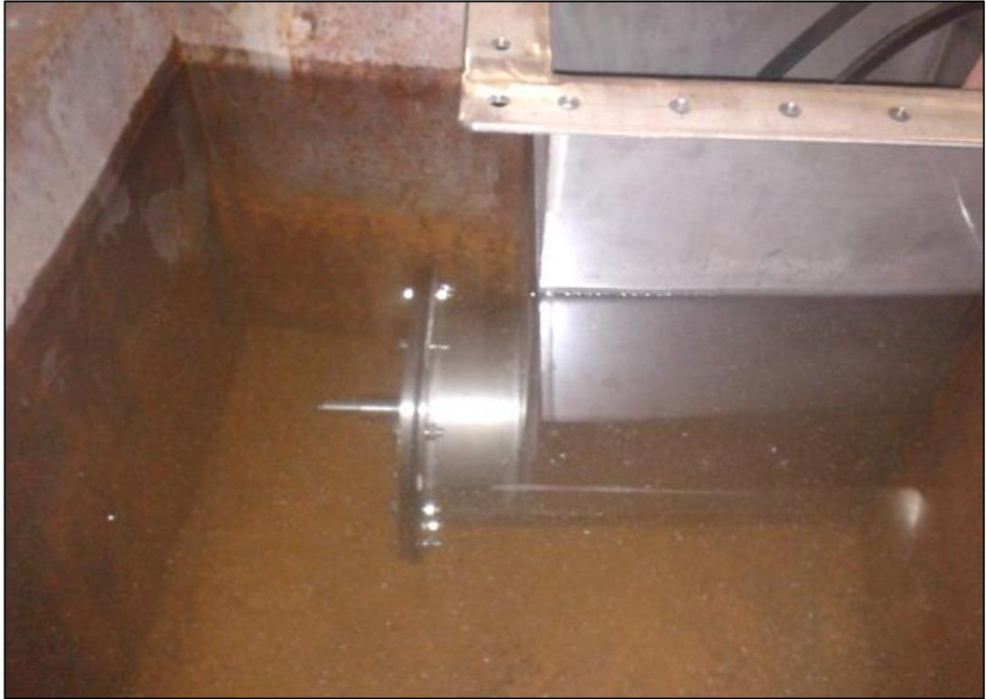
**Figure3.9:** Bottom casing submerged in water to test the suitability of mechanical seal-1.
