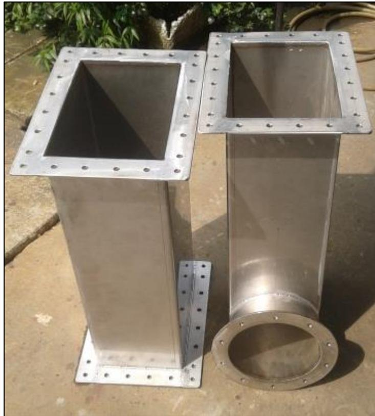
**Figure 3.4:** Bottom casing (right) and top casing (left) of the small scale HATCT.
