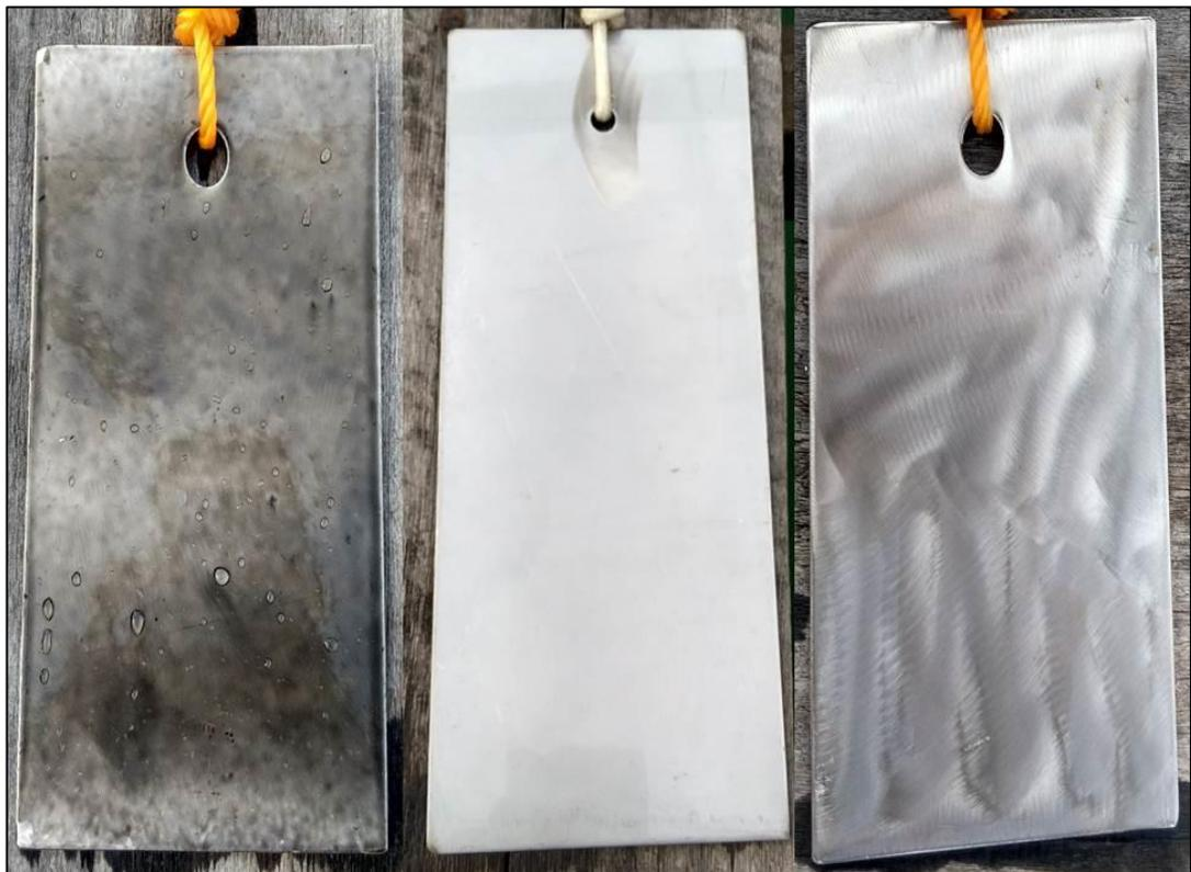
**Figure 4.26:** Stainless steel plates for marine bio-fouling test after 1 day, left (Biocyl), centre (Palccoat) and right (plain).
