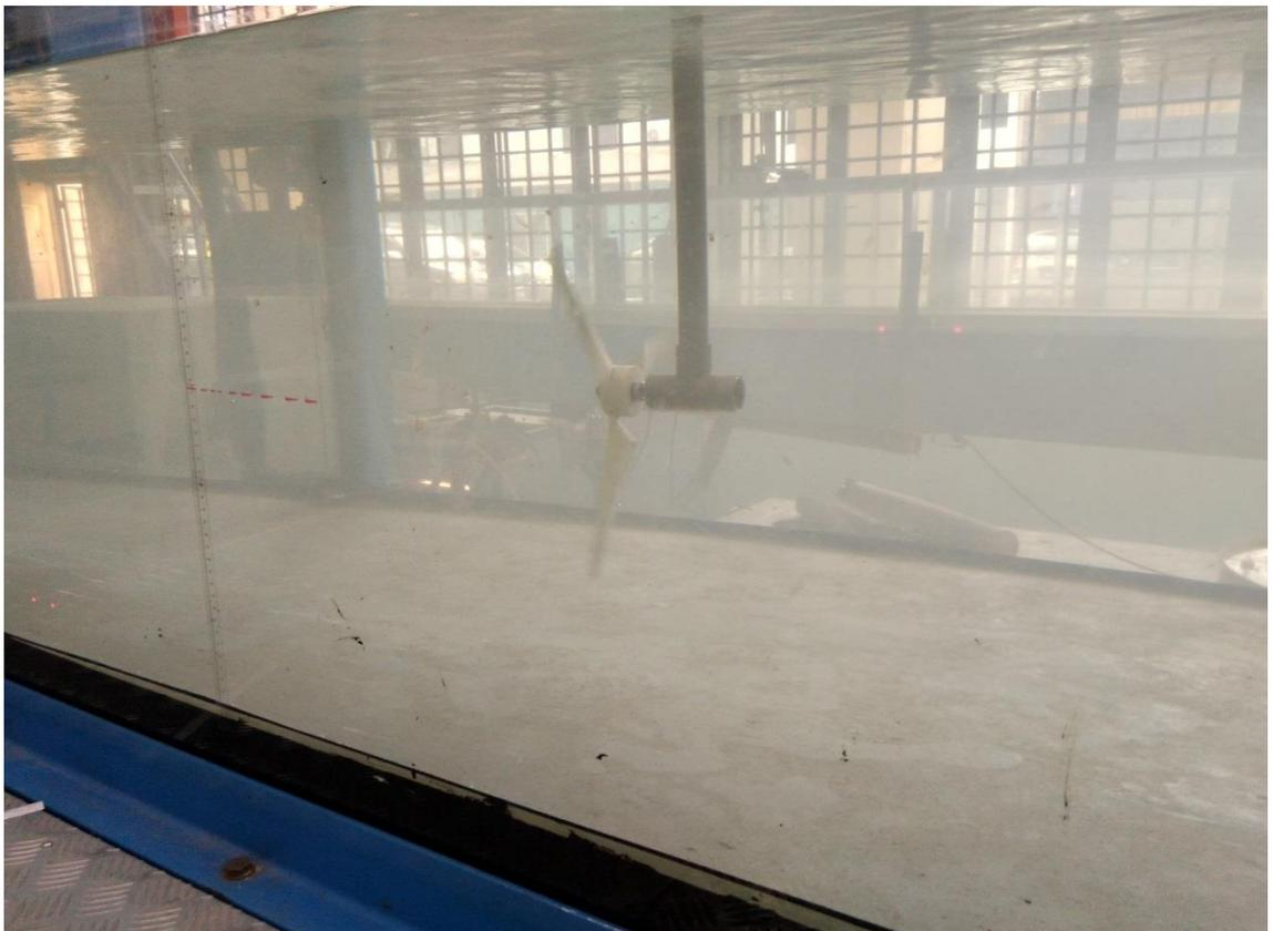
**Fig B4.** Photo taken for lab-scale three-bladed turbine (back)
