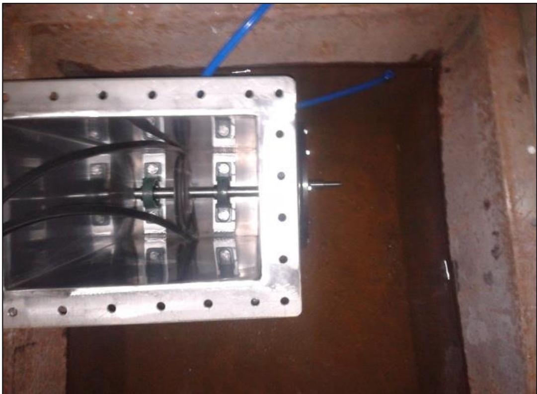
**Figure 3.10:** Bottom casing submerged in water to test the suitability of mechanical seal -2.
