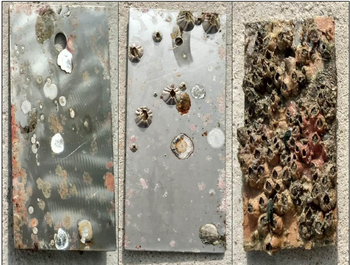
**Figure 4.28:** Cleaned stainless steel plates for marine bio-fouling, left (Biocyl), centre (Palccoat) and right (plain).
