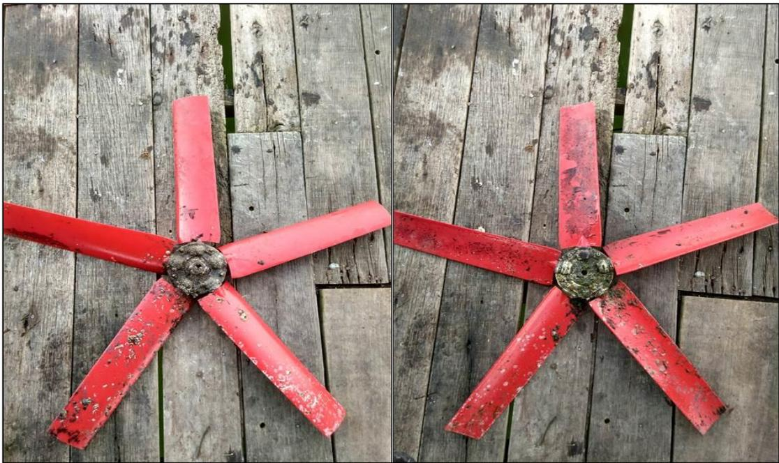
**Figure 4.34:** The FBT after marine fouling test, left (front), right (back).
