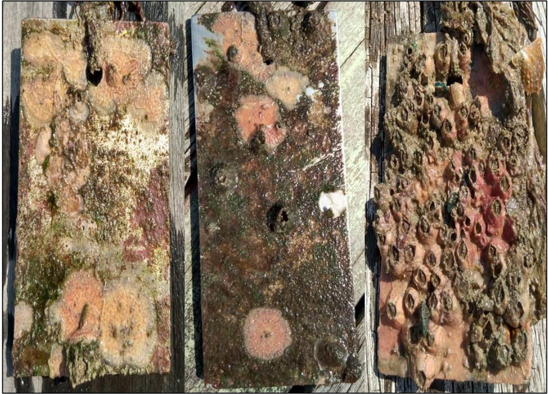
**Figure 4.27:** Stainless steel plates for marine bio-fouling after 90 days, left (Biocyl), centre (Palccoat) and right (plain).
