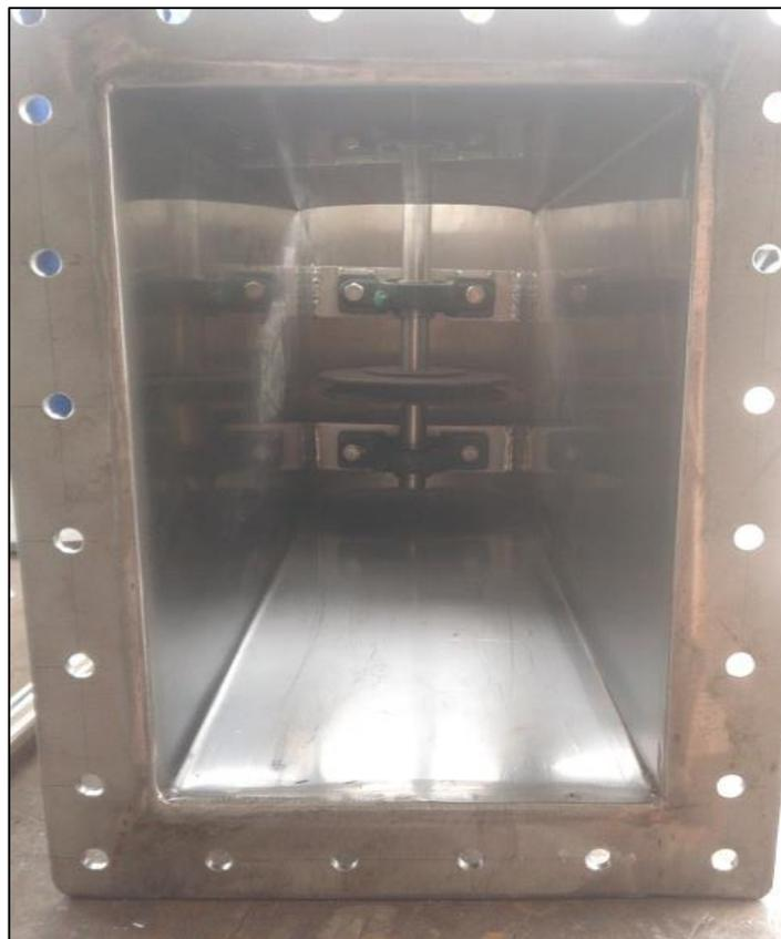
**Figure 3.5:** Plan view of bottom casing of the small scale HATCT with shaft, pulley and bearings.
