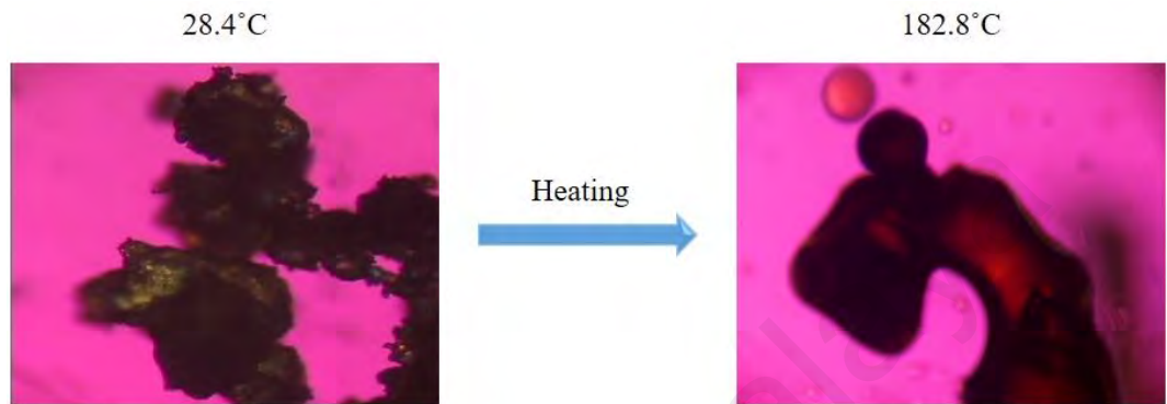
Figure 4.7: Polarizing micrograph of lecithin at 28.4 °C and 182.8 °C.
