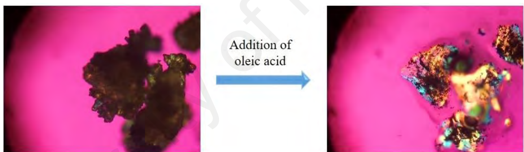
Figure 4.8: Polarizing micrograph of lecithin before and after addition of oleic acid.
