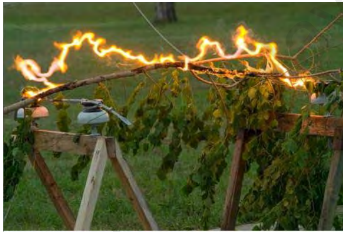
Figure 2.3: An electric arcing phenomenon ( http://phys.org/news/2010-11-faults-vegetation-contact-lines.html#jCp )
