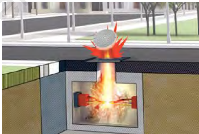
Figure 2.3: An electric arcing phenomenon ( http://phys.org/news/2010-11-faults-vegetation-contact-lines.html#jCp )
