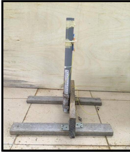
**Figure 3.5:** Pier model made of PVC pipe
