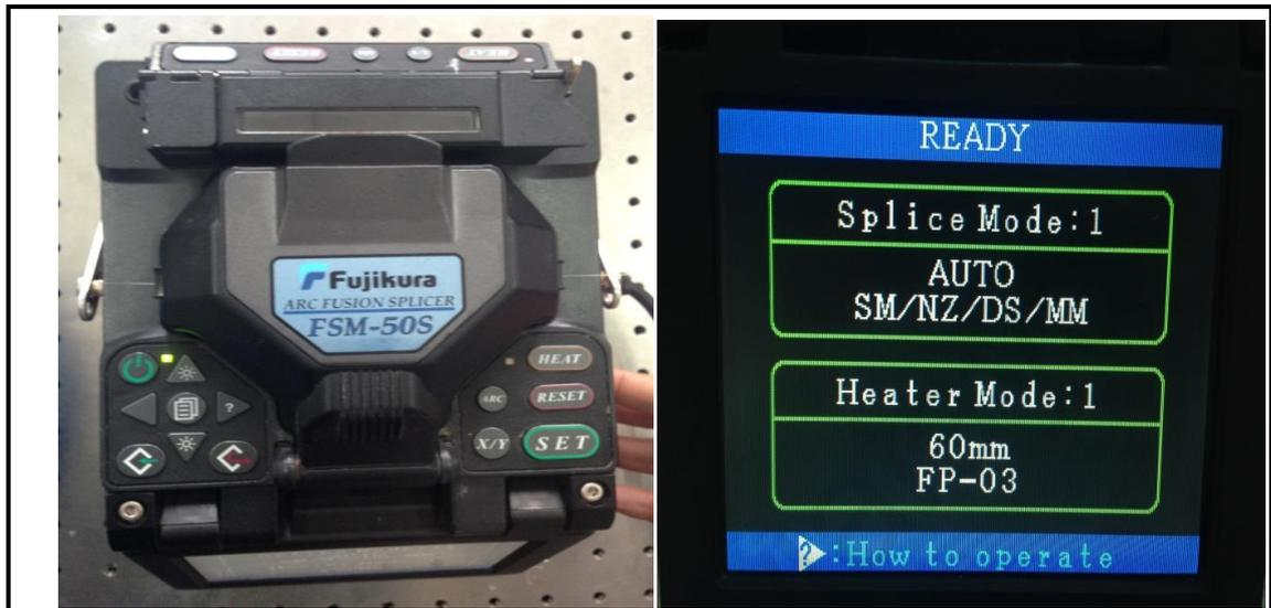
**Figure 3.3: Fujikura Arc Fusion Splicer (a) outside view (b) screen view**
