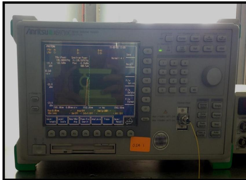
**Figure 3.4: Anritsu Optical Spectrum Analyzer used in this work**
