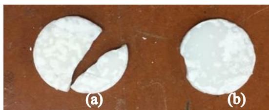
**Figure 4.7: Physical inspection for (a) microwave and (b) conventional samples sintered at 1500 °C after 100 hours of ageing.**
