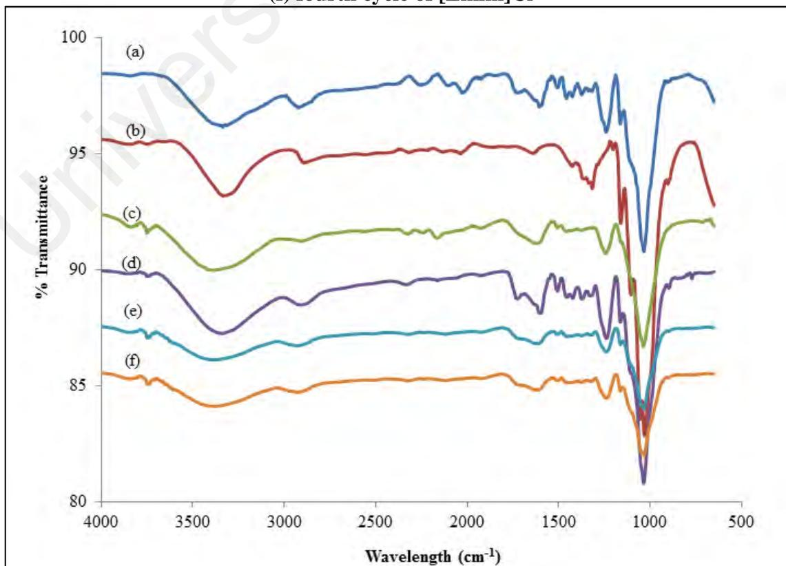
**APPENDIX D 3- FTIR analysis of (a) untreated coconut shell, (b) microcrystalline cellulose and regenerated cellulose from (c) first recycle, (d) second, (e) third and (f) fourth cycle of [Bmim]Cl**
