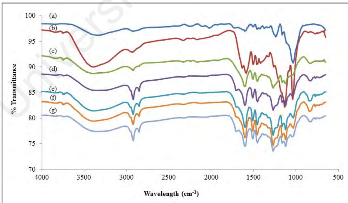
**APPENDIX C 3- FTIR analysis of (a) untreated coconut shell, (b) Kraft lignin and regenerated lignin by (c) fresh IL, (d) first recycle, (e) second, (f) third and (g) fourth recycled [Bmim]Cl**
