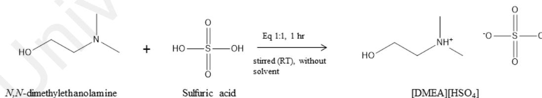
The base was initially placed in a three-necked flask and equipped a dropping funnel. An equimolar amount of sulfuric acid (100.82 g, 0.74 mol) was then added dropwise to the *N,N*-dimethylethanolamine (65.96 g, 0.74 mol) while stirring rapidly in an ice bath. The mixture was stirred for 1 h and yielded the colorless liquid as final product: (99.4 g,
