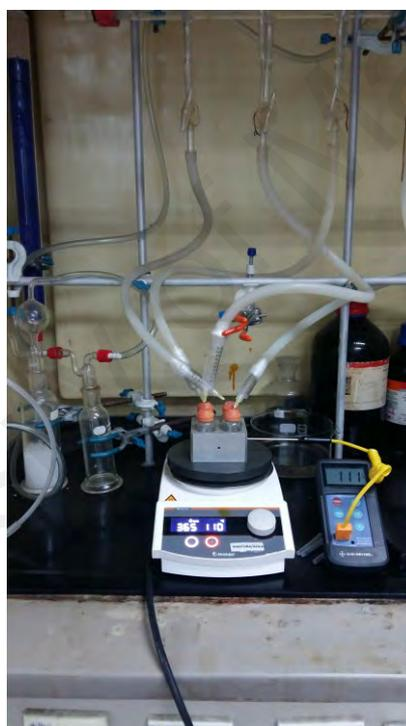
**Figure 3.1: The dissolution process of coconut shell in ionic liquids under a  $N_2$  atmosphere**
