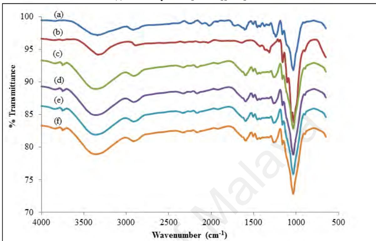
**APPENDIX D 2- FTIR analysis of (a) untreated coconut shell, (b) microcrystalline cellulose and regenerated cellulose from (c) first recycle, (d) second, (e) third and (f) fourth cycle of [Emim]Cl**
