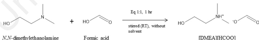
The base was initially placed in a three-necked flask and equipped a dropping funnel. An equimolar amount of formic acid (34.0 g, 0.74 mol) was then added dropwise to the *N,N*-dimethylethanolamine (65.96 g, 0.74 mol) while stirring rapidly in an ice bath. The mixture was stirred for 1 h and yielded the colorless liquid as final product: (99.5 g,
