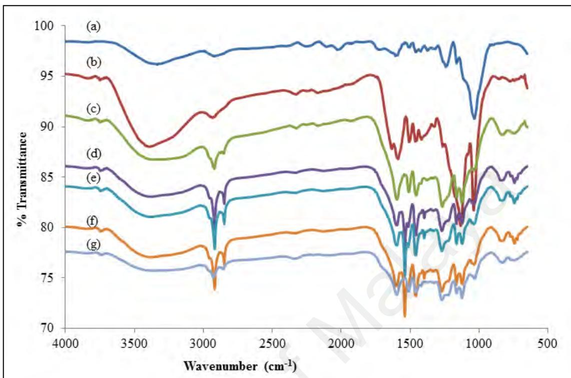
**APPENDIX C 2- FTIR analysis of (a) untreated coconut shell, (b) Kraft lignin and regenerated lignin by (c) fresh IL, (d) first recycle, (e) second, (f) third and (g) fourth recycled [Emim]Cl**
