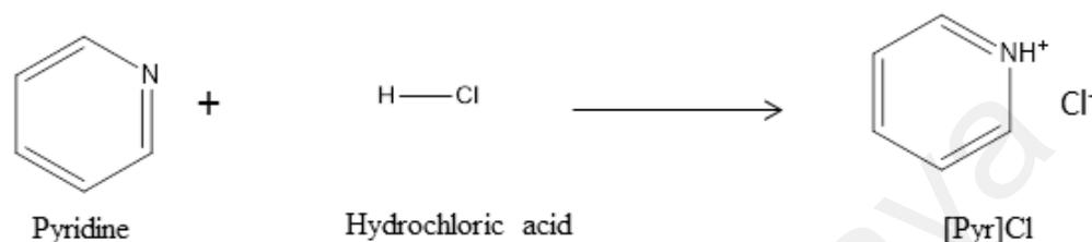
The base was initially placed in a three-necked flask and equipped a dropping funnel. An equimolar amount of hydrochloric acid (74.0 g, 0.74 mol) was then added dropwise to the pyridine (5.87 g, 0.74 mol) while stirring rapidly in an ice bath. The mixture was stirred for 1 h and yielded the colorless liquid as final product: (99.4 g, 99.4 %). <sup>1</sup>H NMR (ppm, 400 MHz, DMSO-d<sub>6</sub>)  $\delta$ H: 8.85 (2H, d, CH), 8.64 (1H, t, CH), 8.09 (2H, t, CH).
