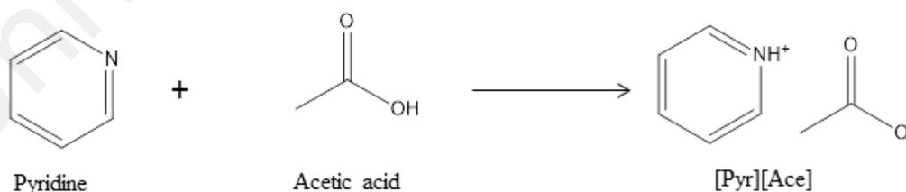
The base was initially placed in a three-necked flask and equipped a dropping funnel. An equimolar amount of acetic acid (51.95 g, 0.74 mol) was then added dropwise to the pyridine (5.87 g, 0.74 mol) while stirring rapidly in an ice bath. The mixture was stirred for 1 h and yielded the colorless liquid as final product: (99.2 g, 99.2%).  $^1\text{H}$  NMR (ppm,
