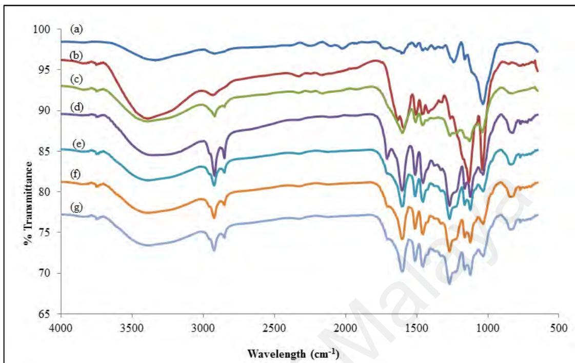
**APPENDIX D 1- FTIR analysis of (a) untreated coconut shell, (b) microcrystalline cellulose and regenerated cellulose from (c) first recycle, (d) second, (e) third and (f) fourth cycle of [Bmim][Ace]**
