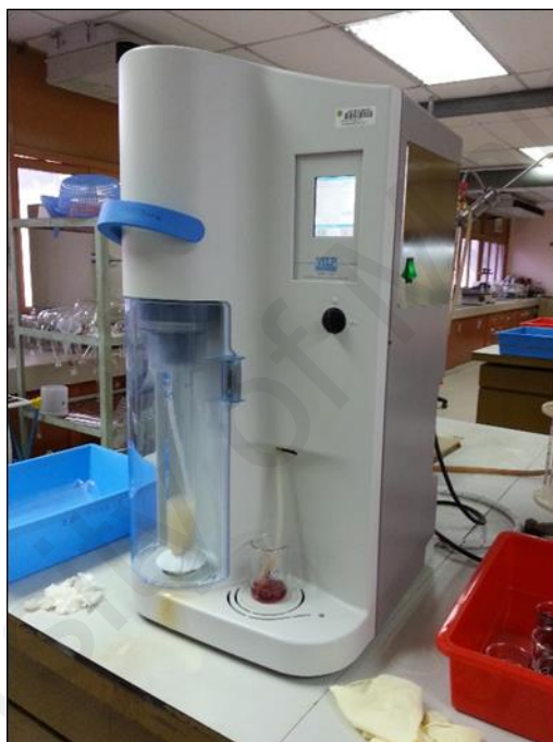
Figure 3.8: Kjeldahl distillation unit
