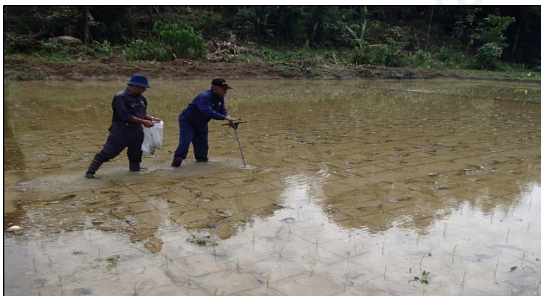
Figure 3.7: Researcher using an auger to pull out soil from identified depth
