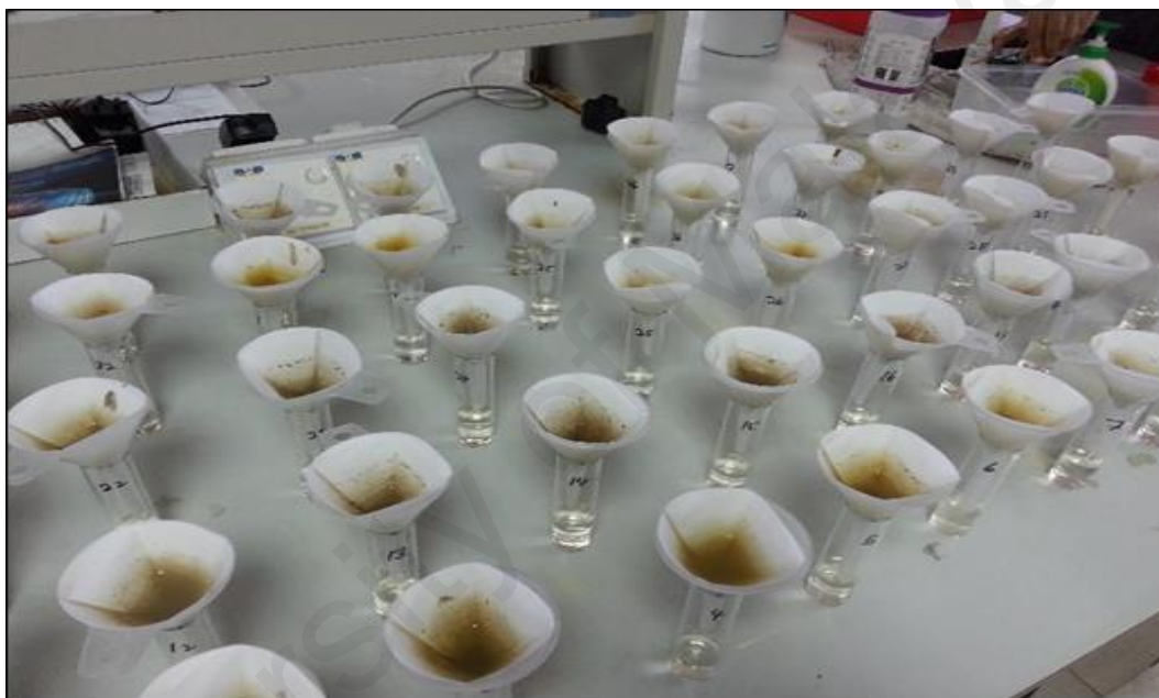
Figure 3.9: Extraction process of soil for phosphorus test
