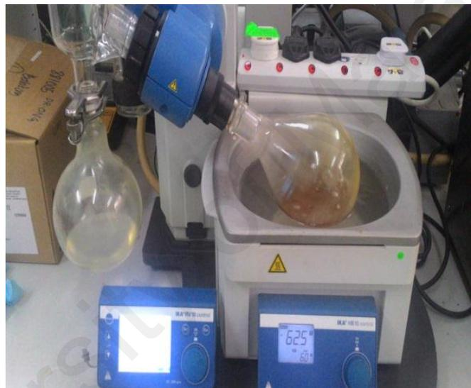
(c) The rotary evaporator equipment used to evaporate extra methanol in biodiesel
