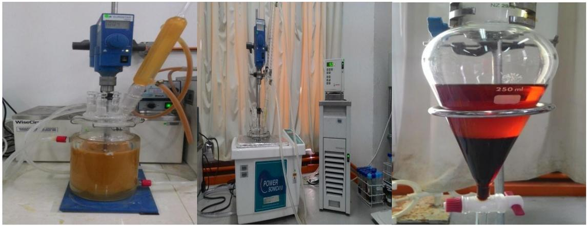
(b) The equipment used for the transesterification process and biodiesel oil on the separation funnel
