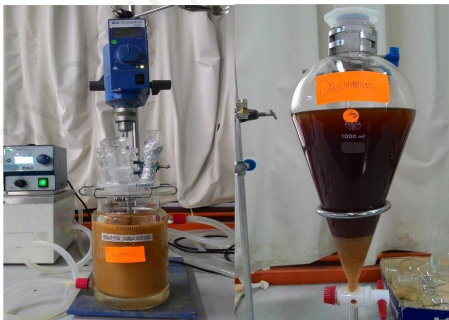
Figure 3.4: Degumming process of *Reutealis trisperma* oil
