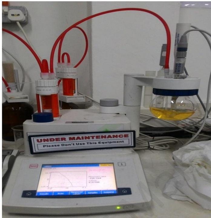
Equipment: Automation titration rondo 20 (Mettler Toledo, Switzerland)
