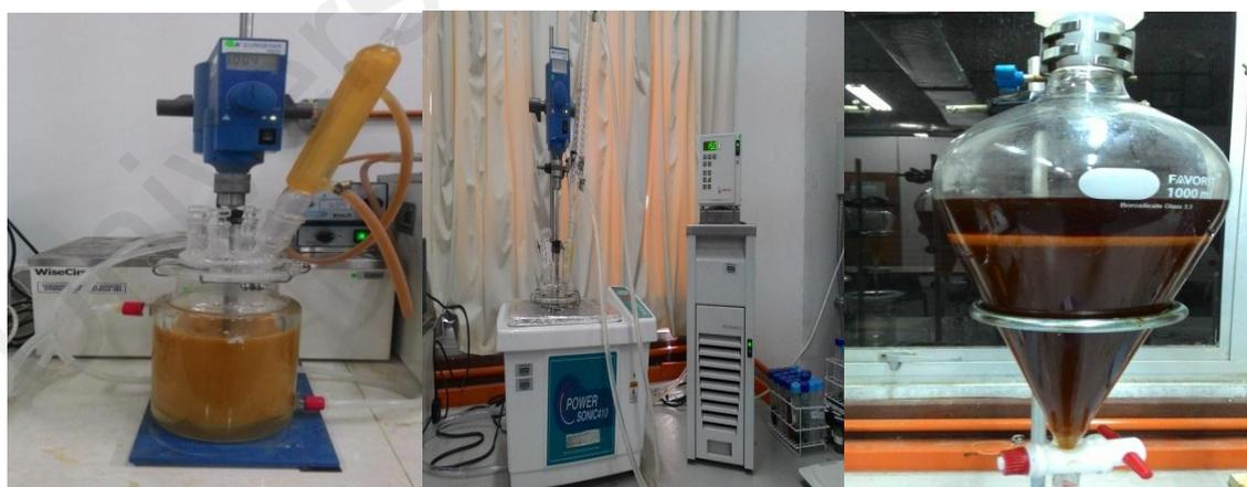
(a) The equipment used for esterification process and esterified oil on the separation funnel
