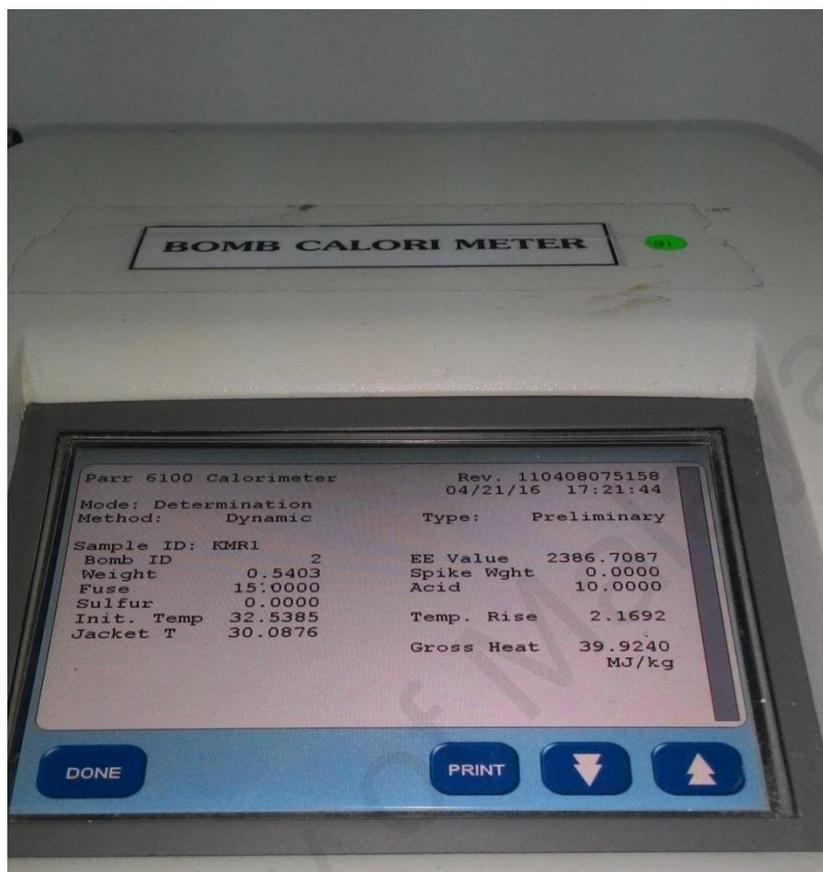
Equipment: 6100EF Semi auto bomb calorimeter (Perr, USA)
