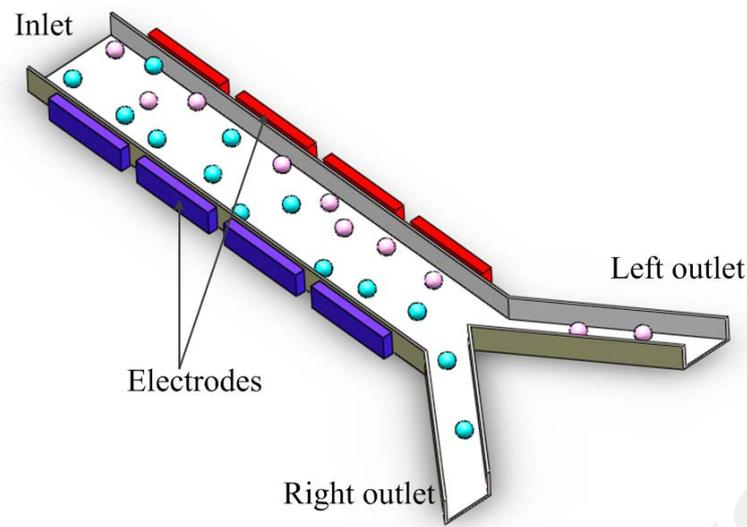
**Figure 2.5: Schematic diagram of the microchip for particle separation based on bi-layer electrodes (reproduced from (Qian *et al.*, 2014))**
