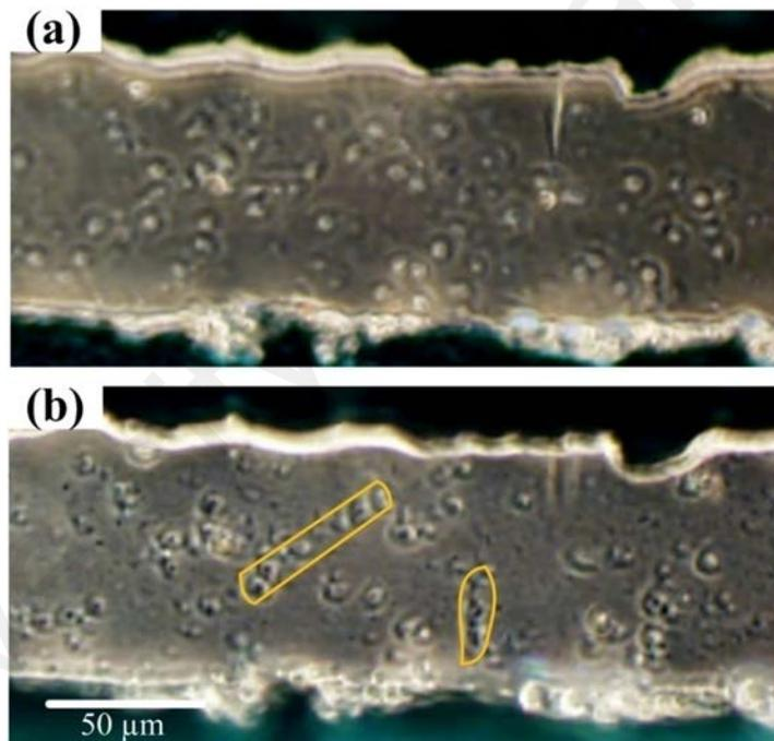
**Figure 5.4: Microscopic images of a cell culture solution with cardiac fibroblasts of density of 106 cells ml<sup>-1</sup> in the microchannel of a fabricated PMMA-based DEP microfluidic chip (magnification of 20×). (a) Before applying a sinusoidal signal to the DEP chip; (b) Applying an AC voltage of 20 V<sub>pp</sub> with frequency of 1 MHz to the two Ag electrodes of DEP chip for 5 minutes.**
