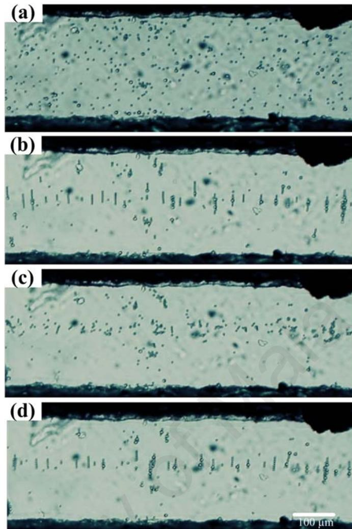
**Figure 5.3: Microscopic images of a suspension with a 5  $\mu\text{m}$ - and 10  $\mu\text{m}$ -diameter PS beads mixture in the microchannel of a fabricated PMMA-based DEP microfluidic chip (magnification of 10 $\times$ ). (a) Before applying a sinusoidal signal to the DEP chip; (b) Applying an AC voltage of 20  $V_{pp}$  with frequency of 1 MHz to the two Ag electrodes of DEP chip; (c) After switching off the applied signals; (d) Re-applying the sinusoidal signals to the electrodes.**
