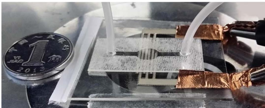
**Figure 4.5: A fabricated DEP microfluidic chip placed on microscope stage. A Chinese coin of 10 cent with diameter of 18 mm was placed besides the DEP chip for size comparison.**
