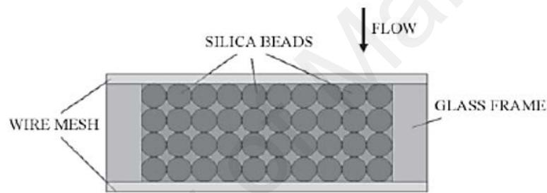
**Figure 2.2: A schematic of 3-D DEP filter using silica beads (adapted from (Tay et al., 2009))**
