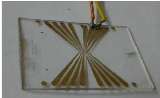
**Figure 2.3: The gold coated planar electrode.**
