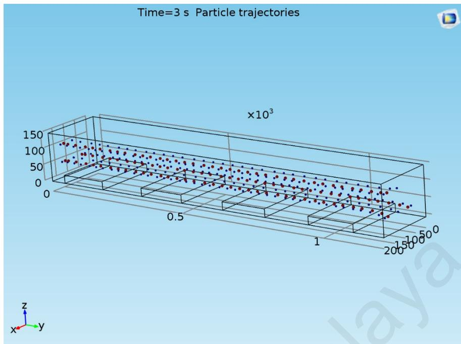
**Figure 3.3: Figure showed the distribution of particle flowing in the micro channel with the DEP deactivated. Red dots represent the red blood cells while blue dot represent the platelets.**
