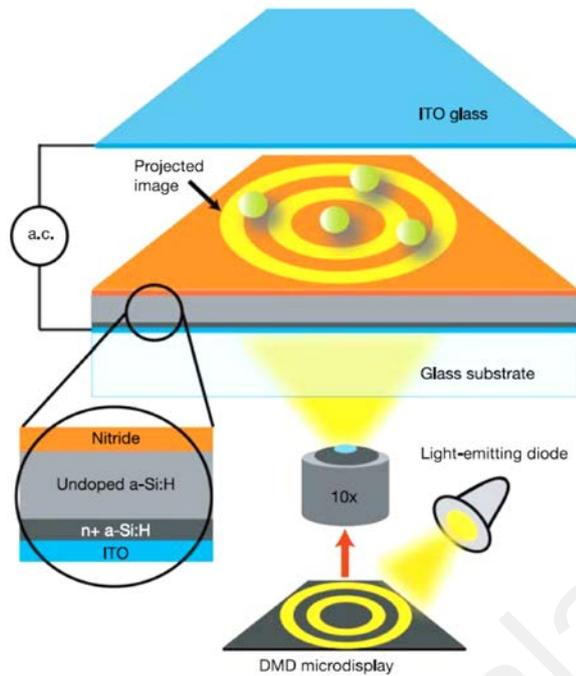
**Figure 2.6: Device structure used in optoelectronic tweezers. Liquid that contains microscopic particles is sandwiched between the top ITO glass and the bottom photosensitive surface consisting of ITO-coated glass topped with multiple featureless layers (adapted from (Pei Yu Chiou *et al.*, 2005))**
