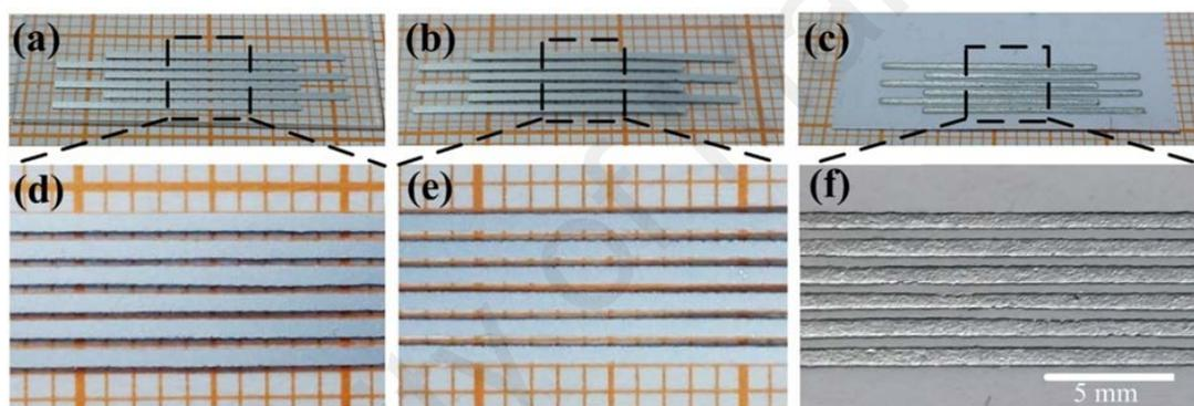
**Figure 4.3: (a-c) Photographs and (d-f) microscopic images of the Ag electrode patterns printed on different substrates: (a,d) a PMMA substrate, (b,e) a PET substrate, and (c,f) an A4 paper substrate. The background substrates are the graph papers with squares of 1 mm x 1 mm (length x width).**
