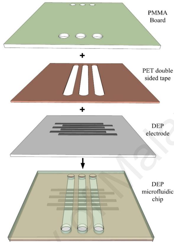
**Figure 4.4: The schematic diagram of the fabrication of DEP microfluidic chip**
