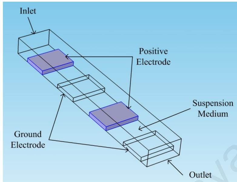
**Figure 3.2: 3D model of the electrode setup used in determine the factors.**
