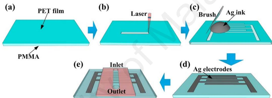
**Figure 4.2: Schematic of the fabrication process of a DEP microfluidic chip on a PMMA substrate**
