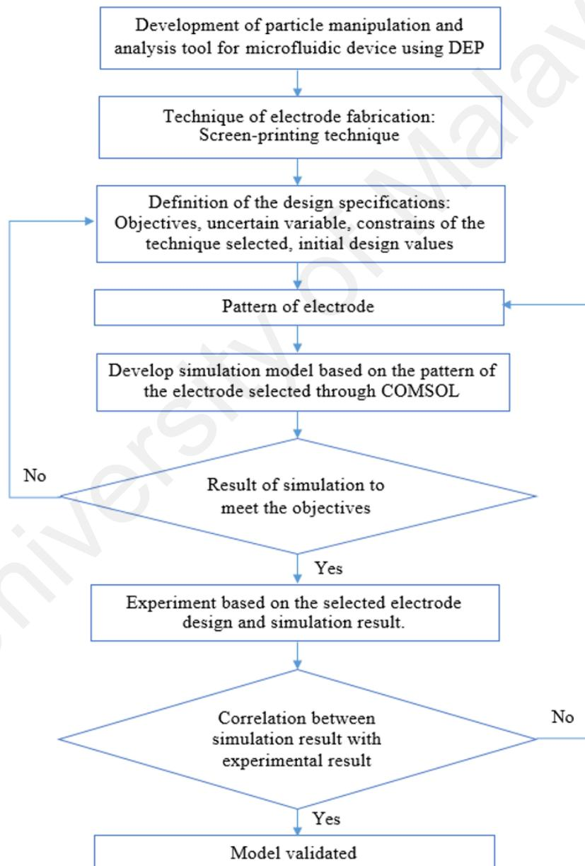
**Figure 3.1: The flow chart illustrating the design specifications and validation process for the electrode of the DEP microfluidic chip.**
