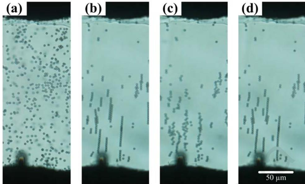
**Figure 5.2: Microscopic images of a 3  $\mu\text{m}$ -diameter PS beads suspension in the microchannel of a fabricated PMMA-based DEP microfluidic chip (magnification of 40 $\times$ ). (a) Before applying a sinusoidal signal to the DEP chip; (b) Applying an AC voltage of 20 Vpp with frequency of 1 MHz to the two Ag electrodes of DEP chip for 5 minutes; (c) After switching off the applied signals; (d) Re-applying the sinusoidal signals to the electrodes.**
