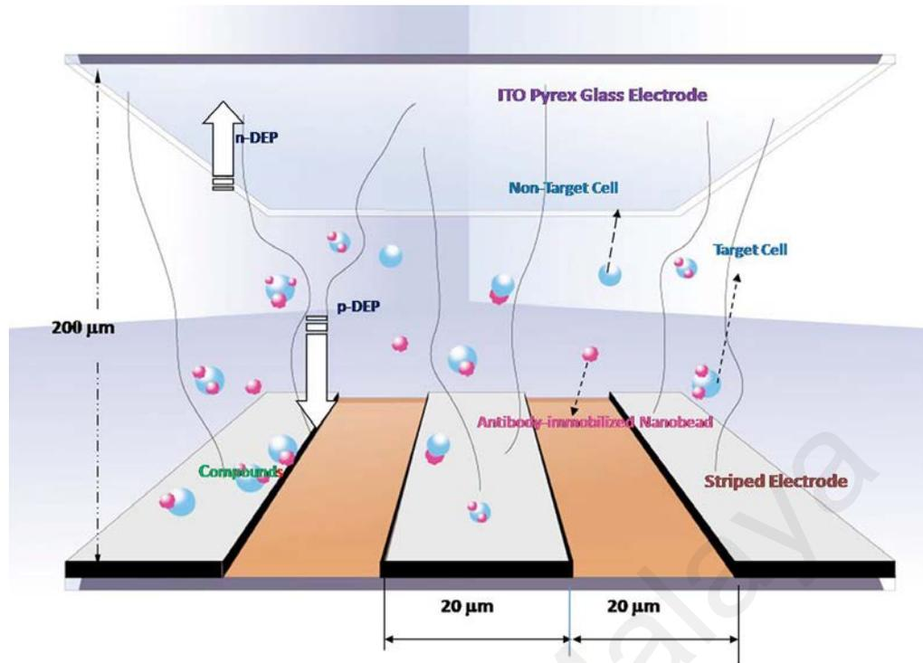
**Figure 2.4:** The mixture of normal cells and nanobeads attached cells were subjected to DEP field between bi-layer electrode formed by ITO Pyrex glass and striped electrode. Target cells were trapped on stripped electrode and separated out from the mixture (reproduced from Wang, 2009).
