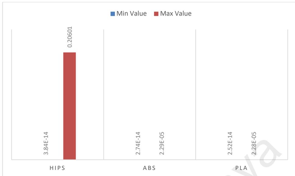
**Figure 4.19 Maximum and Minimum values of different materials for Equivalent Elastic Strain**
