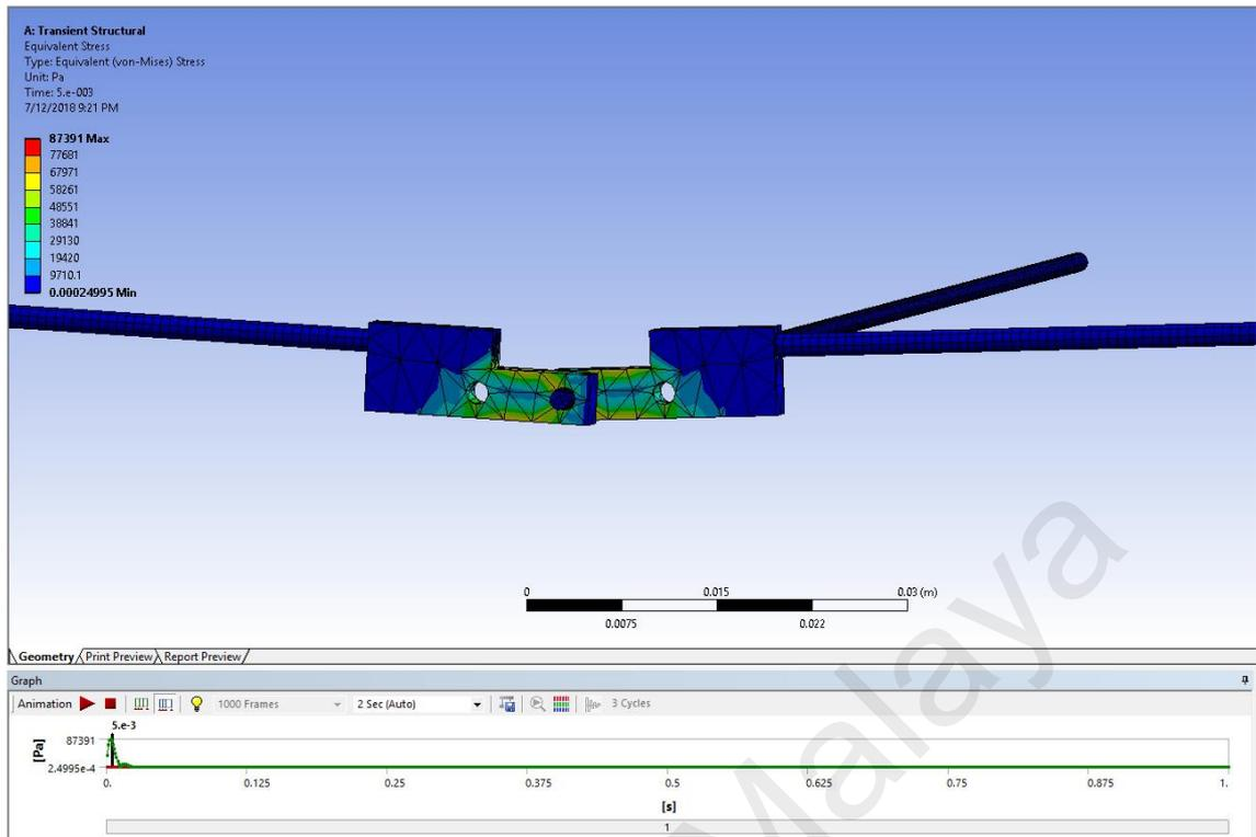
Figure 4.7 Equivalent Stress
