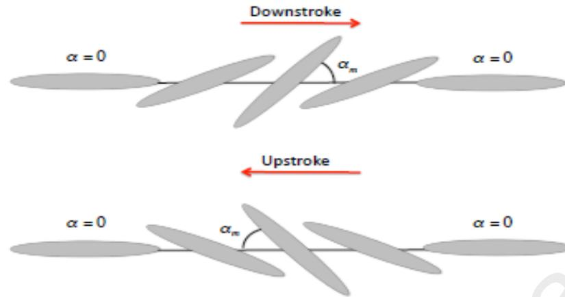
**Figure 2.3 Upstroke and Downstroke of a wing, when  $\alpha=0^\circ$**
