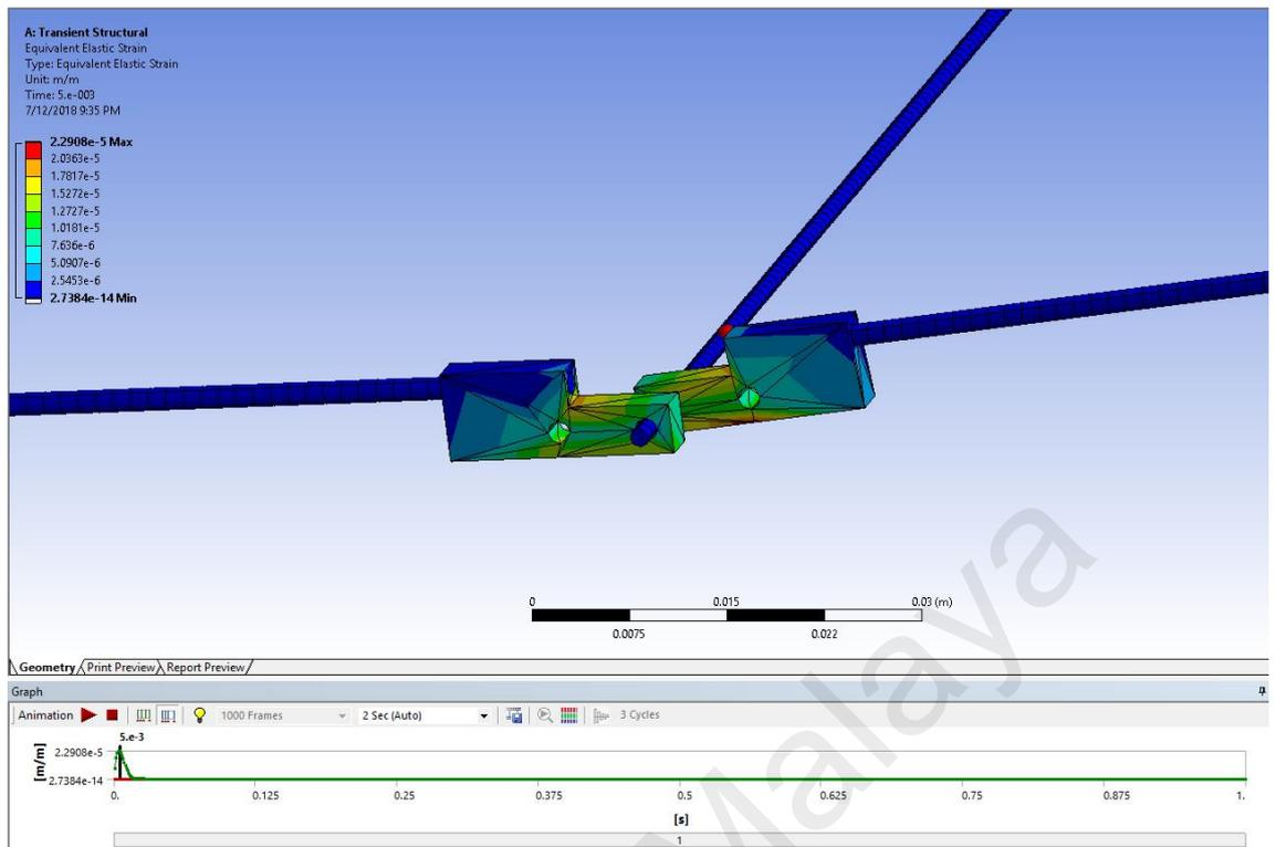
**Figure 4.11 Equivalent Elastic Strain**
