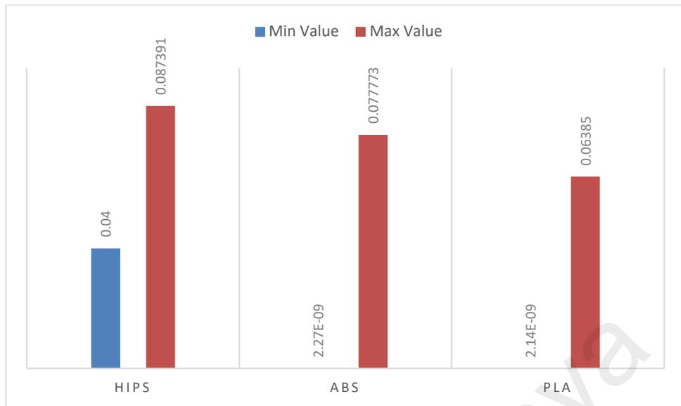
**Figure 4.20 Maximum and Minimum values of different materials for Equivalent Stress**
