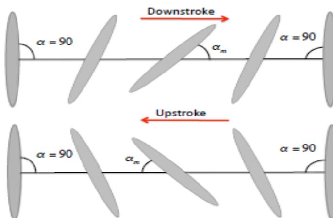
**Figure 2.2 Upstroke and Downstroke of a wing, when  $\alpha=90^\circ$**
