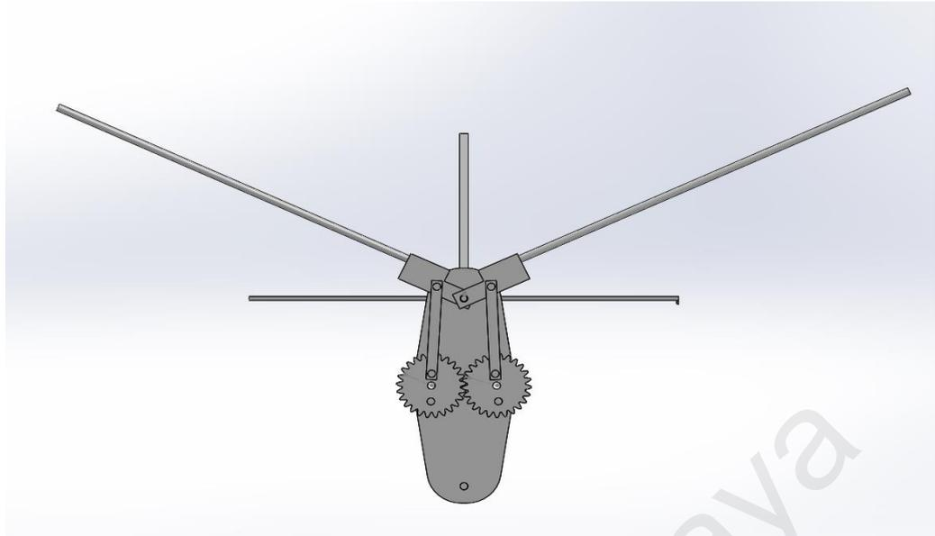
**Figure 4.4.2 Position of the highest flap**
