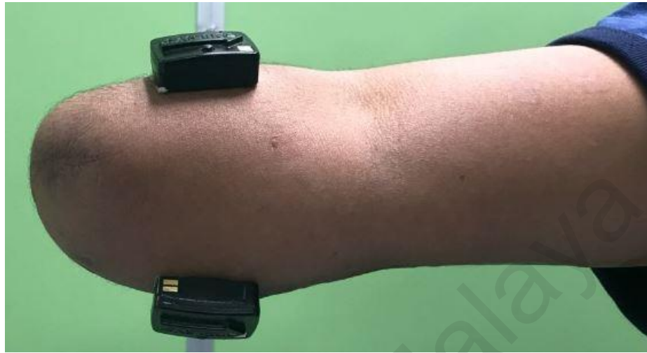
Figure 3.10: Muscles utilized during test two and respective electrode placement of muscles for transradial amputees
