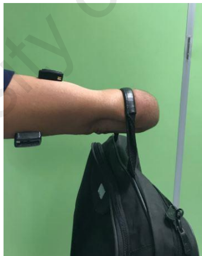
Figure 3.17: Flexion and Extension of the muscles above elbow with 3kg weight for amputee subjects during test 1
