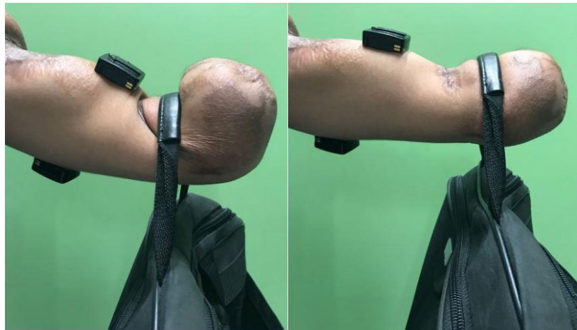
Figure 3.18: Flexion and Extension of the muscles above elbow with 3kg weight for non-amputee subjects during test 1
