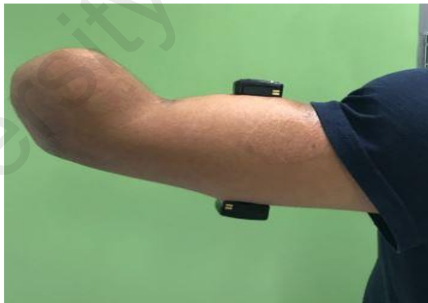
Figure 3.7: Electrode placement site for transradial amputee during test 1
