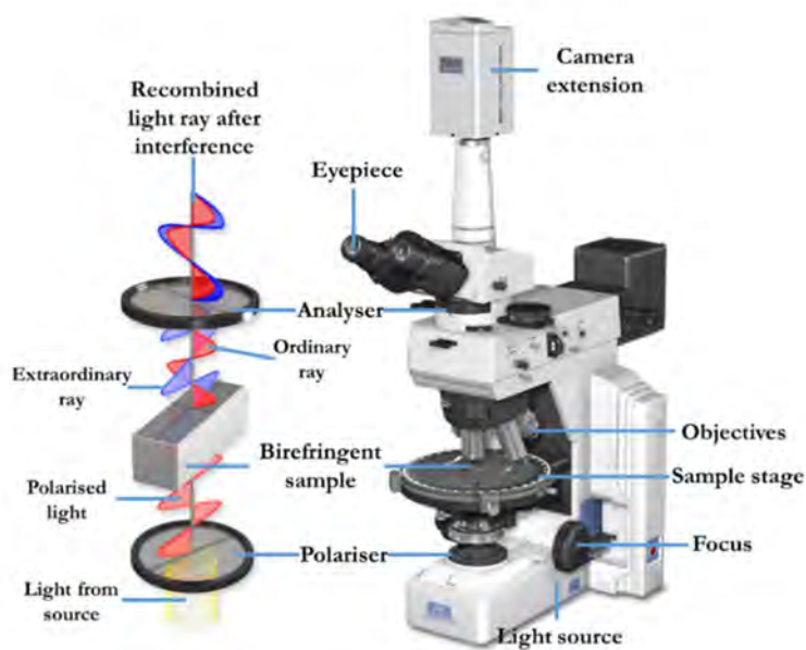
Figure 2.6: Setup of optical polarising microscope. Redrawn from (Robinson & Davidson, 2016).
