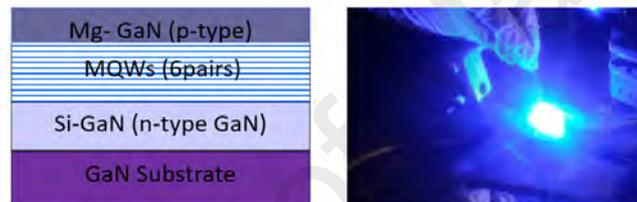
**Figure 5.1: Left: Schematic of GaN-on-GaN LEDs structure , Right: Blue light emission**
