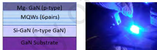
**Figure 3.4: Left: Basic schematic of the GaN-on-GaN blue LEDs structure, Right: Blue light emission**
