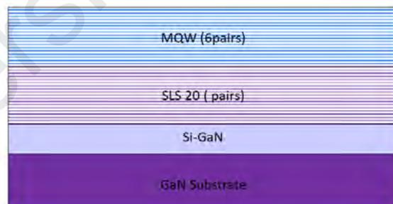
**Figure 4.7: Sample G046, MQWs structure with SLS layer**
