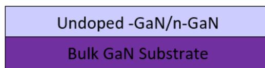
**Figure 4.1: The first layer on bulk GaN substrates**
