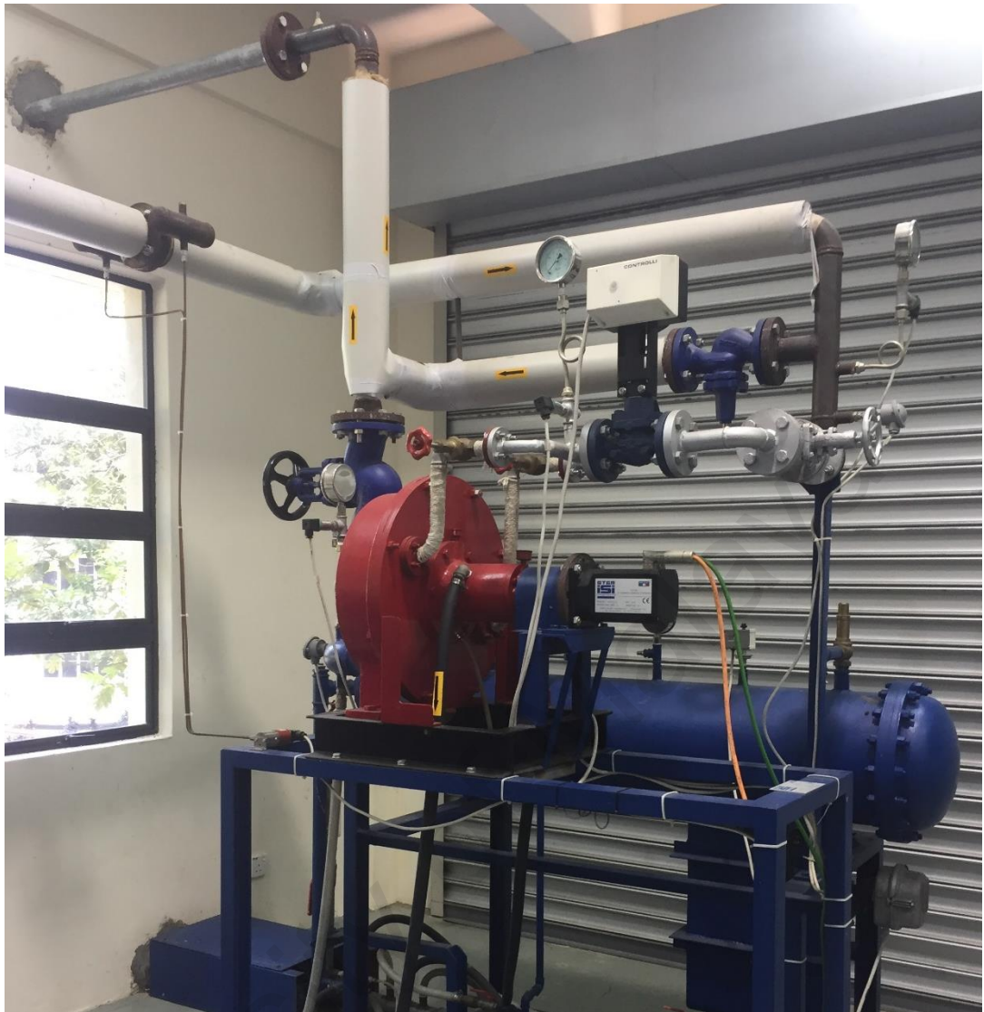
Figure 3.6: Turbine connected through shaft with generator
