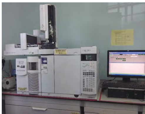
Figure 3.3: GC-FID for analysis of essential oils
