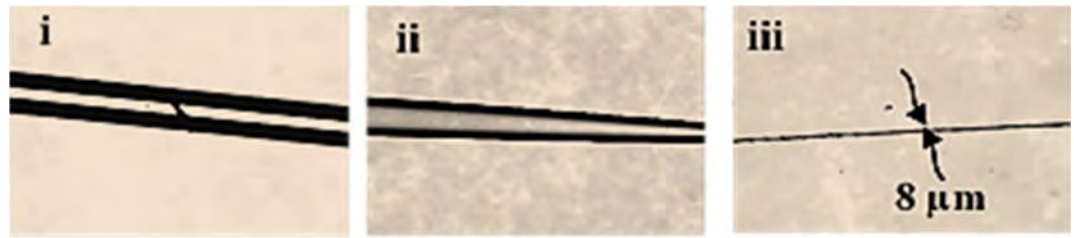
Figure 3.5: View of the fabricated microfiber (i) stripped untapered fiber, (ii) part of the transition region, and (iii) waist region.
