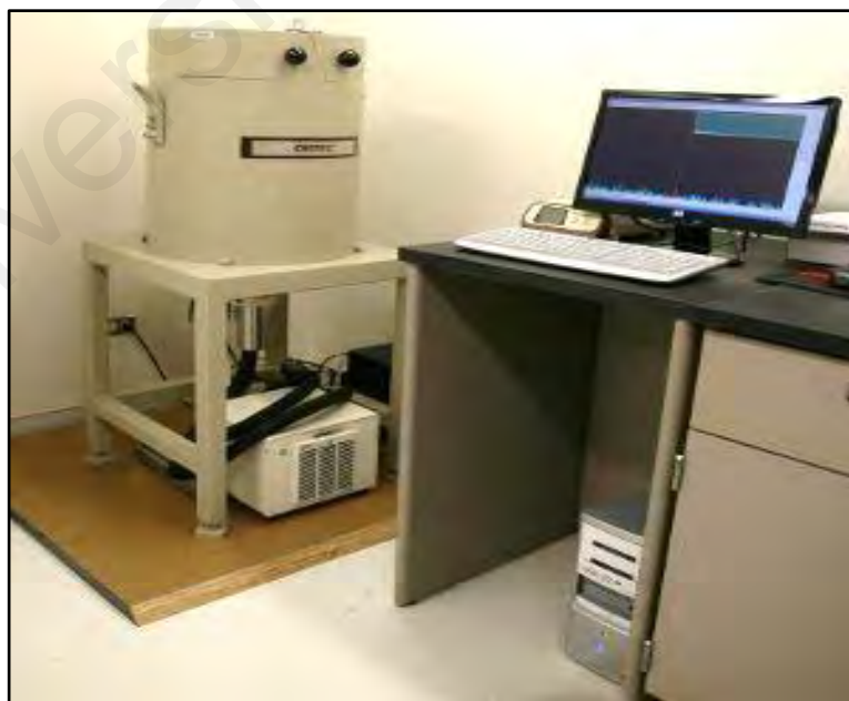
Figure 3.29: High-purity germanium (HPGe) gamma-ray spectrometry machine located at Nuclear Malaysia.
