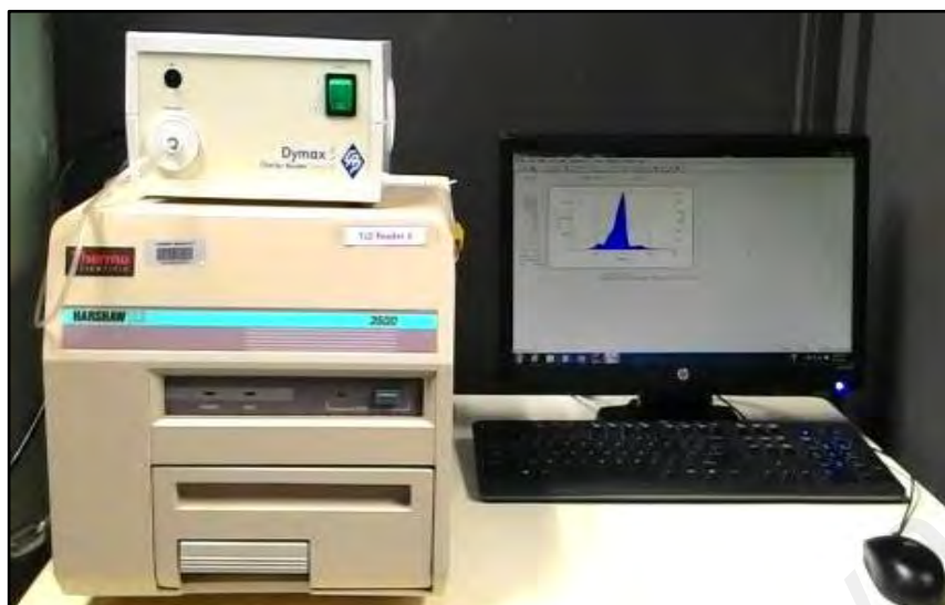
Figure 3.8: A Harshaw 3500 TLD reader, supported by WinREMS software, the vacuum tweezers being used for sample handling.
