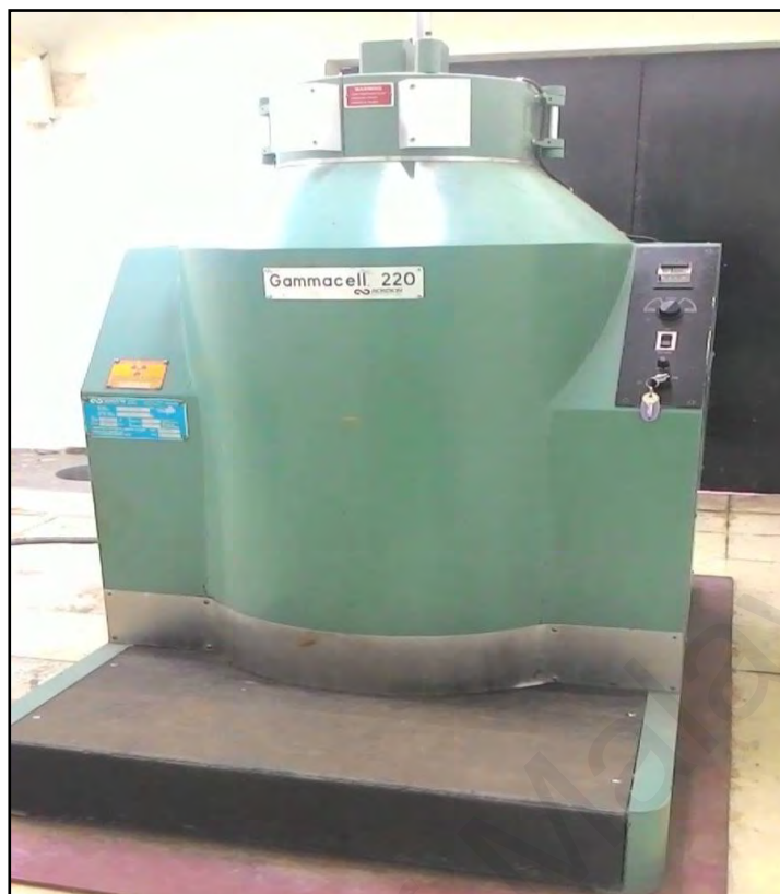
Figure 3.7: A conventional Gammacell-220 ^{60}\text{Co} , located at Department of Physics, University of Malaya.
