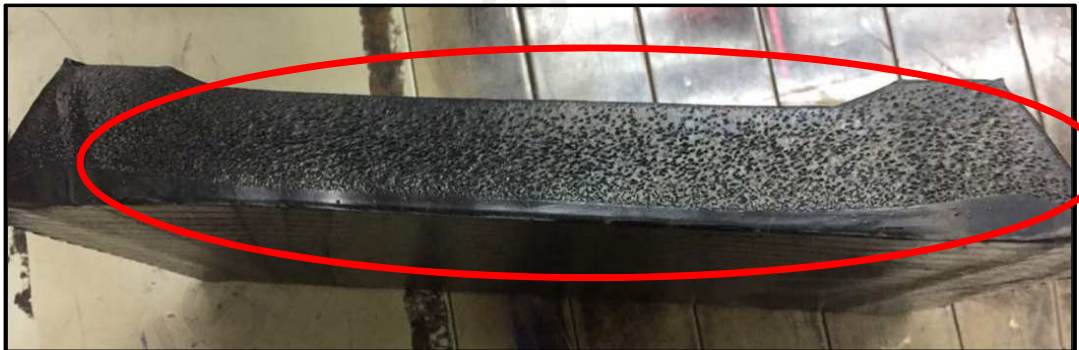
Figure 5.2 Porosity area due to high humidity absorb by rubber compound
