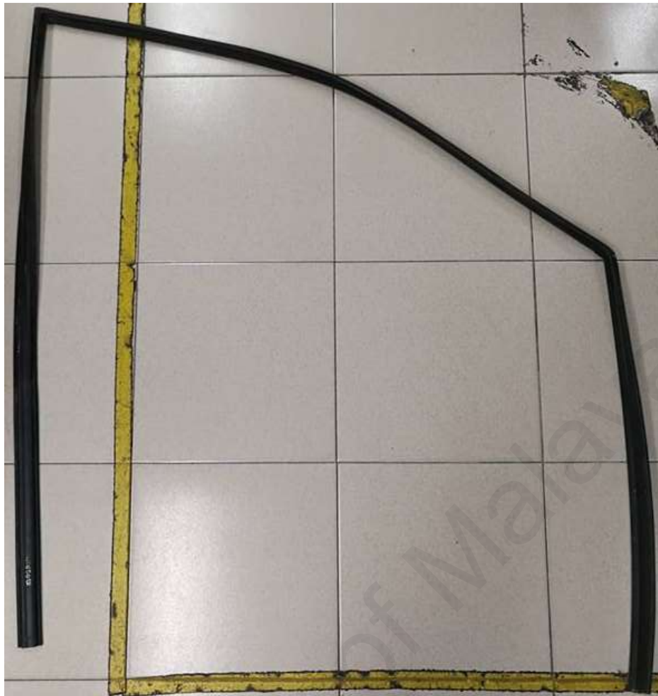
Figure 4:31: Figure above shows the Glass Window Rubber Seal component.
