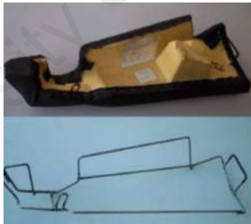
Figure 2.3: Figure above shows the encapsulated steel frame with thermoset by (Sopher, 2009)
