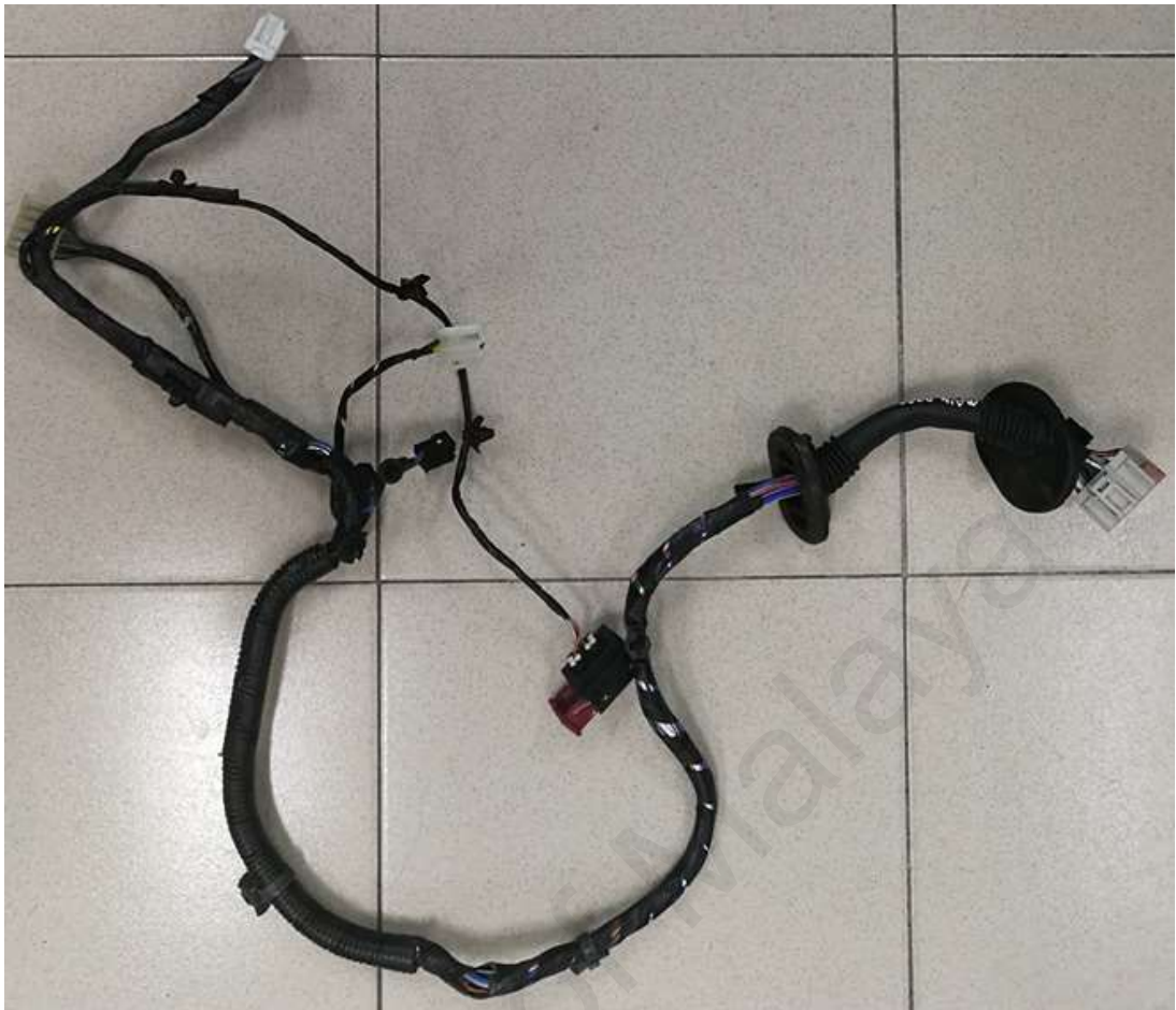
Figure 4:17: Figure above shows the Main Door Wiring subassembly.
