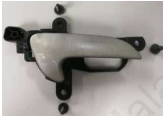
Figure 4:1: Figure above shows a sub-assembly of an Interior Door Handle sub-assembly.
