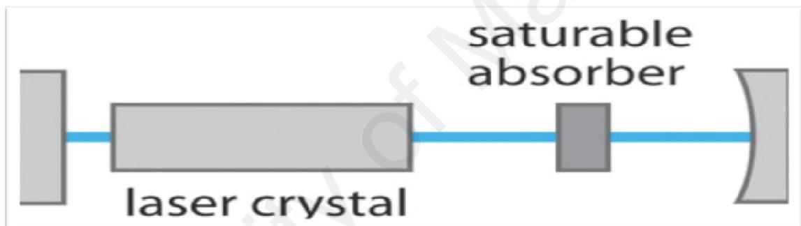
**Figure 2.3: Basic structure of passive Q-switch device**
