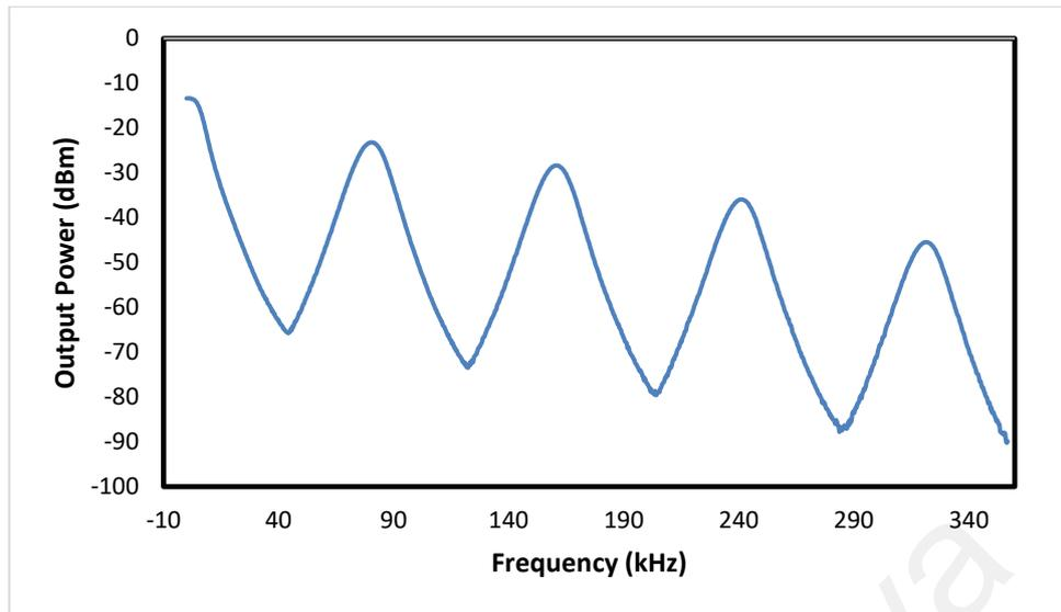
**Figure 4.10. RF spectrum at pump power of 200 mW**
