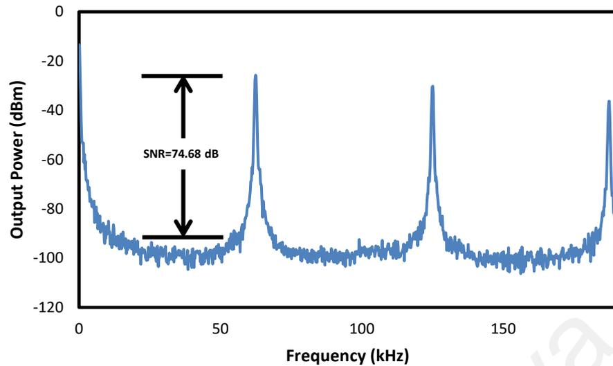
**Figure 4.5: RF spectrum at pump power of -2.49mW**
