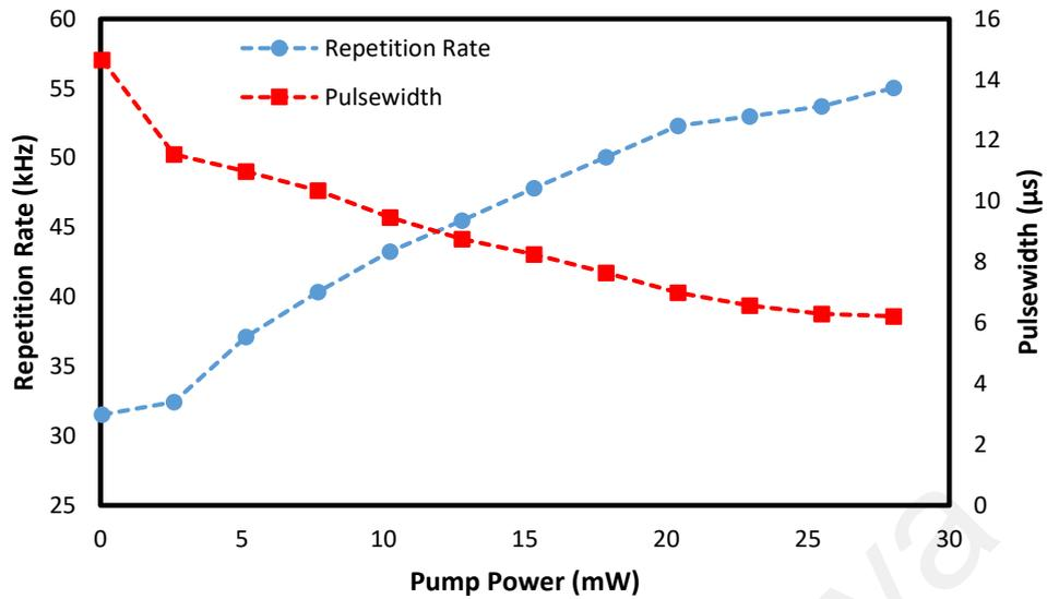
**Figure 4.3: Repetition rate and pulse width as functions of input pump power**
