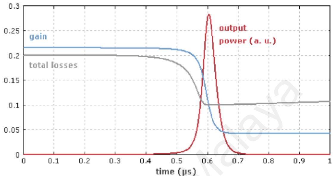
**Figure 2.4: Evolution of gain and losses in a passive Q-switching laser**
