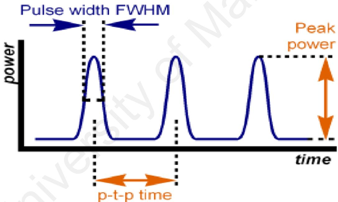
Figure 2.6: Pulse characteristic
