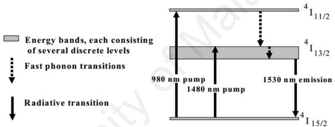
**Figure 2.1: Energy diagram of Erbium ( $Er^{3+}$ ) in silica fibers (Citation)**
