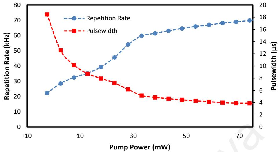
**Figure 4.8: Repetition rate and pulse width as functions of input pump power**
