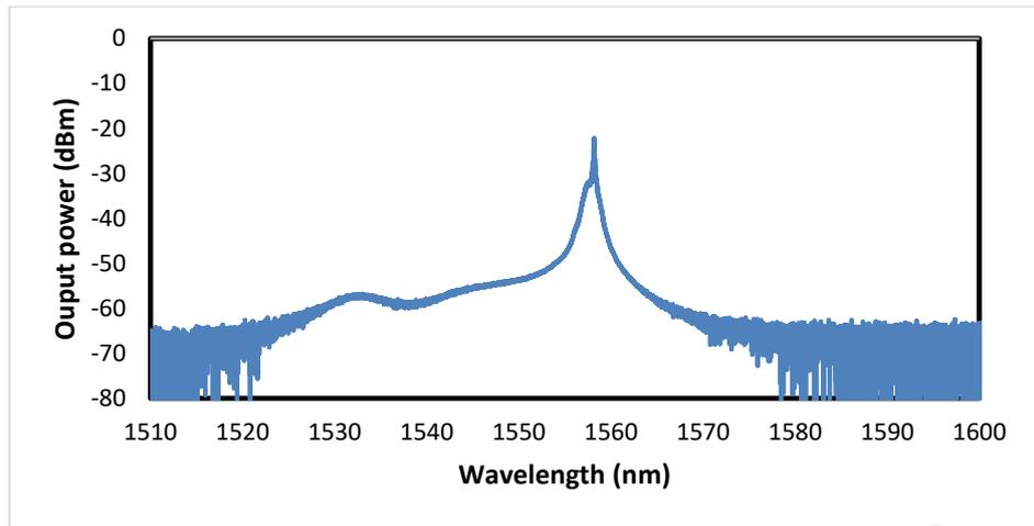
**Figure 4.6: Typical optical spectrum of the proposed Q-switched EDFL at pump power of 28.038 Mw**
