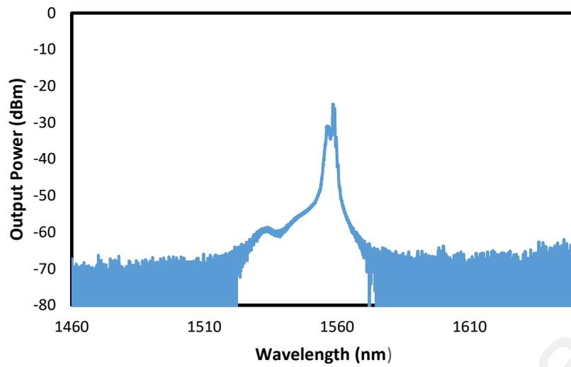
**Figure 4.1: Typical optical spectrum of the proposed Q-switched EDFL at pump power of 28.038 Mw**
