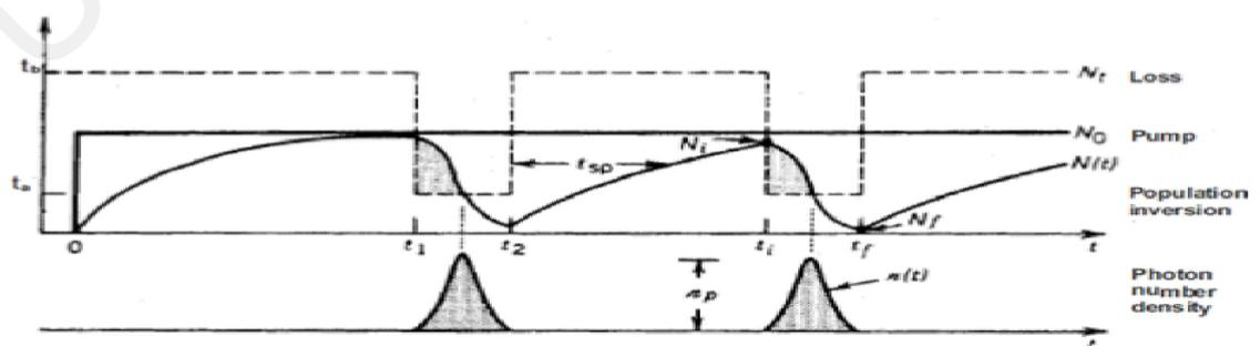
**Figure 2.5: Principle of a Q-switched laser**
