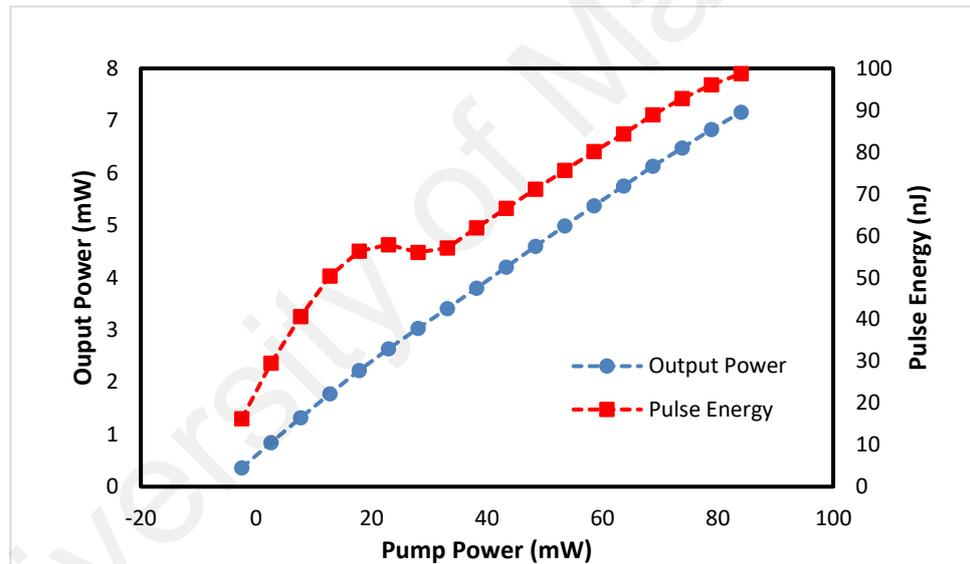
**Figure 4.9: Average output power and single-pulse energy as functions of input pump power**
