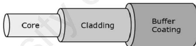
**Figure 2.2: Optical Fiber Layers**
