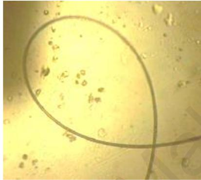
**Figure 3.1: MLR Microscopic image of 5  $\mu\text{m}$  diameter microfiber with its 300  $\mu\text{m}$  diameter loop**
