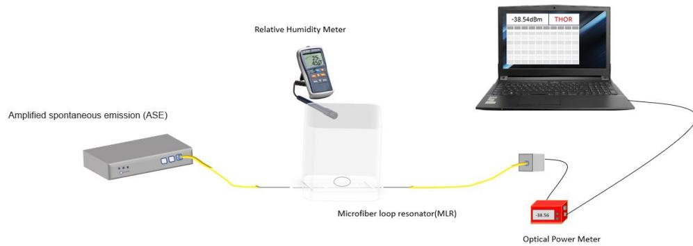
**Figure 3.3: Experimental setup of MLR for taking WGM transmission mode**
