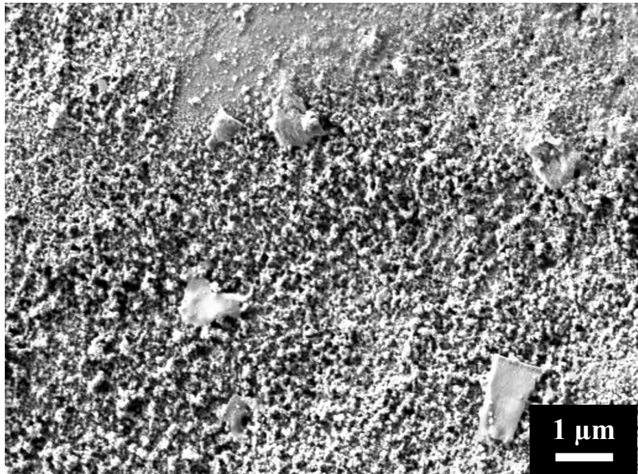
Figure 4.39: Worn surface morphology of SPE implant after 12 weeks of implantation at high magnification (10000×)
