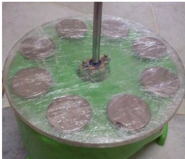
Figure 4.17: Eight-pole single-rotor double-stator assembly.
