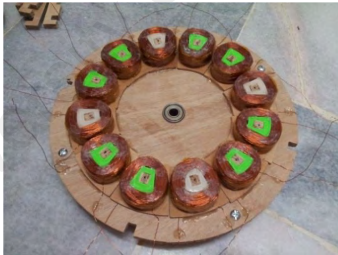
Figure 4.16: Windings configuration for 12-stator core count.
