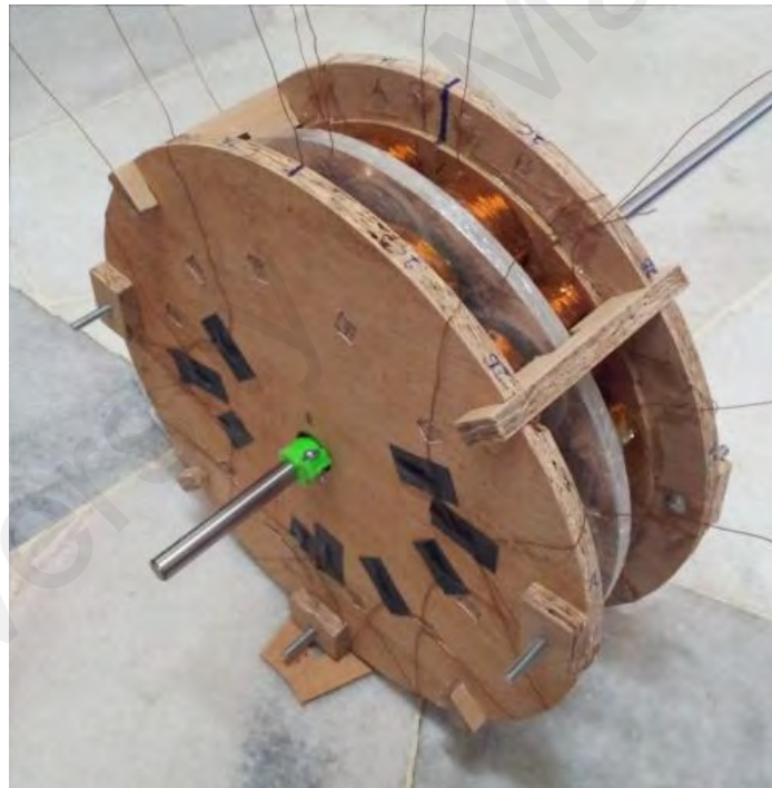
Figure 4.13: Prototype three-phase AFPM machine.
