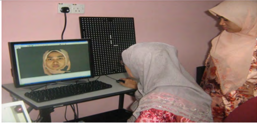
Figure 3.10: The VECTRA-3D Stereo-photogrammetry System: An examiner acquired the 3D facial image of a respondent and performed the anthropometric measurement on the 3D facial image using the Mirror ® Software.
